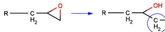
Fig. 2 – Conversion of an original epoxide group to a reactive one through breaking the C-O bond
