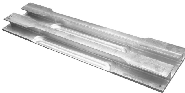
FIG. 3—As-fabricated and machined skin stringer panel.
