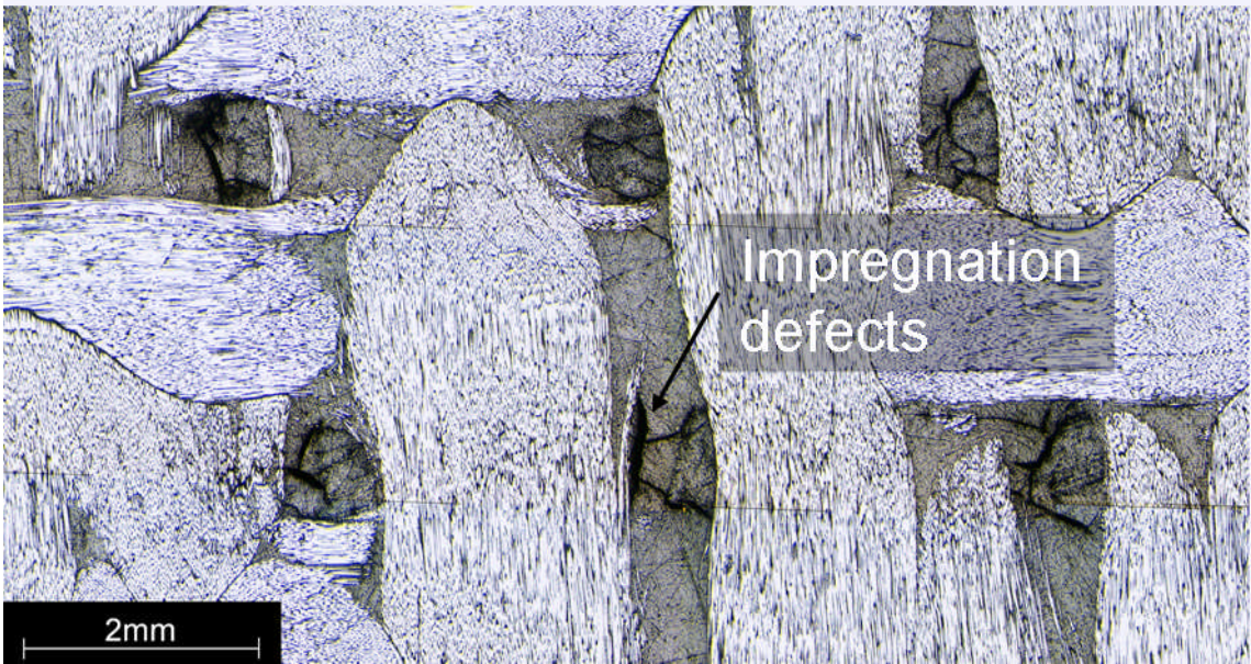
Figure 7: Resin pockets and impregnations defects in a glass thread tufted composite
