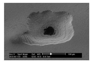
Fig 13. SEM micrograph of a 150  $\mu$ m hole PZT in a 35  $\mu$ m thick PZT film produced using mask with a 110 $\mu$ m aperture. Defect near the bottom left of the hole is due to delamination of the photoresist and subsequent over etch.
