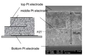
Fig 10. Schematic and SEM image of a multilayer PZT thick film 14[C+4S] with embedded electrode after the 7<sup>th</sup> composite layers.
