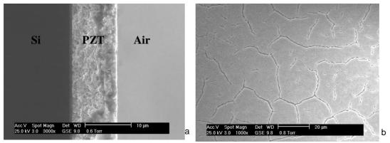
Fig 5. SEM micrograph of 10µm PZT thick film composed of 4[C+4S], cross section (a), surface (b).
