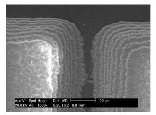
Fig. 11. SEM micrograph of a 21  $\mu$ m PZT thick film, patterned with features at the base of 10  $\mu$ m.
