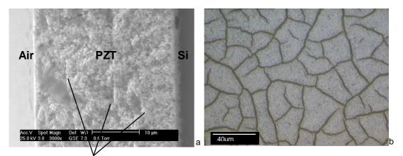
Example of infiltration sol remaining at the interface between two composites layers
