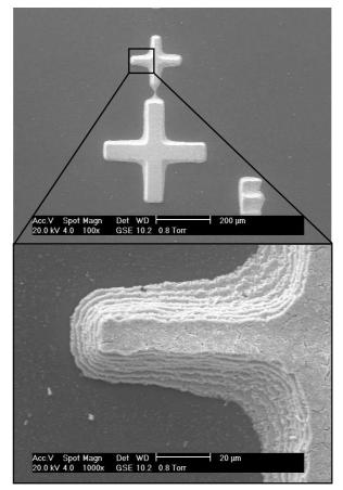
Fig 14. SEM micrograph of a 21  $\mu$ m PZT thick film, patterned to produce a 10  $\mu$ m wide feature
