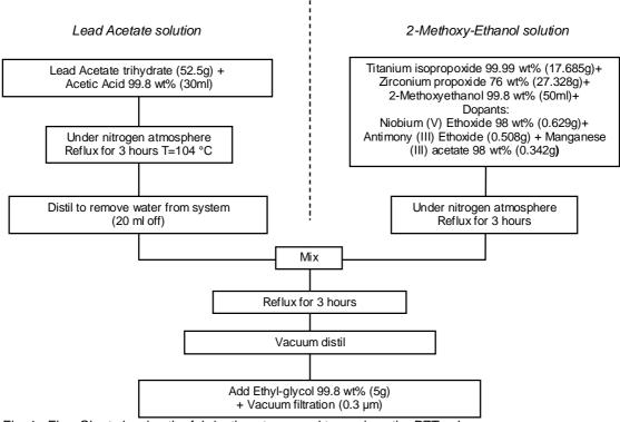
Fig. 1. Flow Chart showing the fabrication steps used to produce the PZT sol
