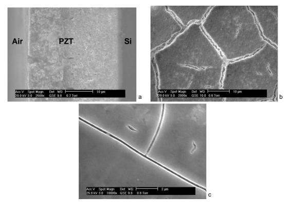
Fig 7. SEM micrograph of  $35\mu$ m PZT thick film composed of 16[C+4S] a) cross section, b) surface, c) surface of the same film coated with 1 layer of pure PZT sol showing reduction in crack width.
