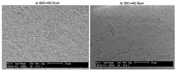
Fig 8. SEM micrograph of surface finish of the process x[2C+4S] for 2 different thicknesses of film showing a marked reproduction in cracking in comparison to x[C+4S] films. a) with 100nm of Pt sputtered the surface, b) virgin PZT surface
