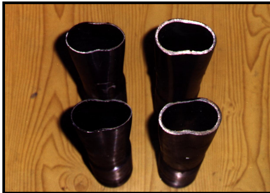
Figure - 3 Typical Post- buckling Configurations in Case of Elastic-Plastic Collapse (X52 and X56 steel pipe specimens after sectioning)
