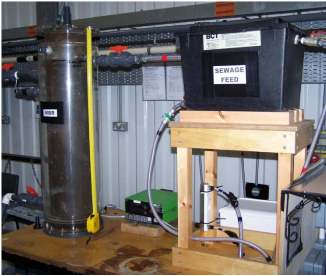
MBR (left) and Sewage feed tank (right)
