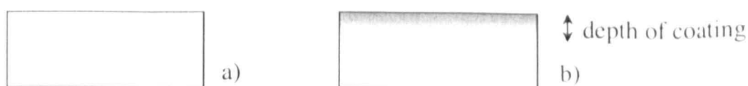
Figure 2-1: Schematic of a component a) uncoated and b) with a diffusion coating.
