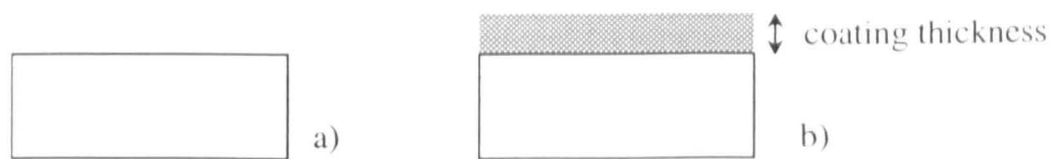
Figure 2-2: Schematic of a component a) uncoated and b) with an overlay coating.
