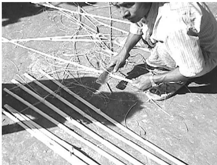
Figure 11: Cutting of Bamboo Slats
