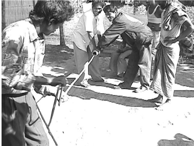
Figure 17: Cleaning the Pith out of the Bamboo
