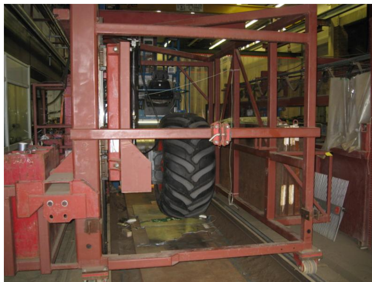
Figure 3.4 The 12 tonne loading frame designed by Ansorge (2005) for large agricultural tyres
