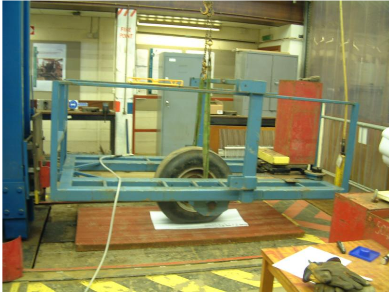
Figure 3.5 The 5 tonne loading frame for medium agricultural tyres attached via a hinged pivot point to the soil processor
