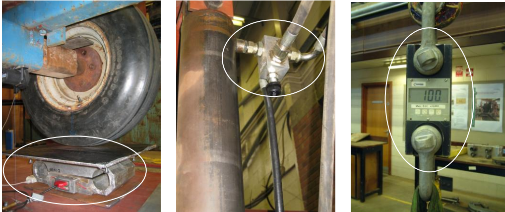
Figure 3.7 Load measuring equipment (left: extended octagonal ring transducer, middle: hydraulic pressure transducer, right: tension link dynamometer)
