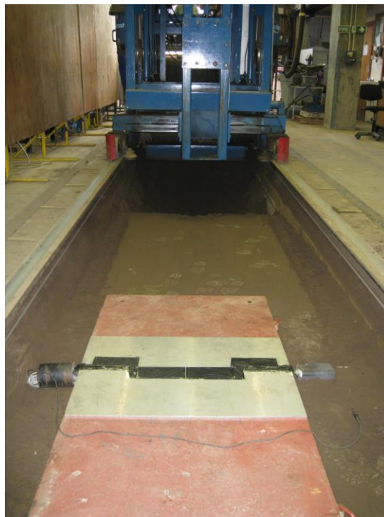
Figure 4.15 The 9830_A and 9830_B Tekscan sensors placed in the soilbin
