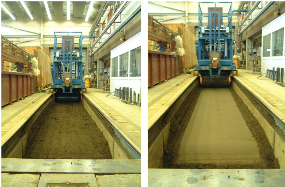
Figure 3.2 Soil preparation in the soil bin (left: soil spreading, right: soil compacting)
