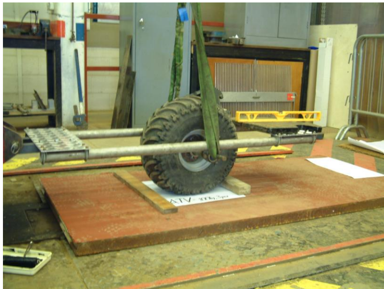
Figure 3.6 The 0.25 tonne loading frame for small agricultural tyres attached via a hinged pivot (far left) to the soil processor
