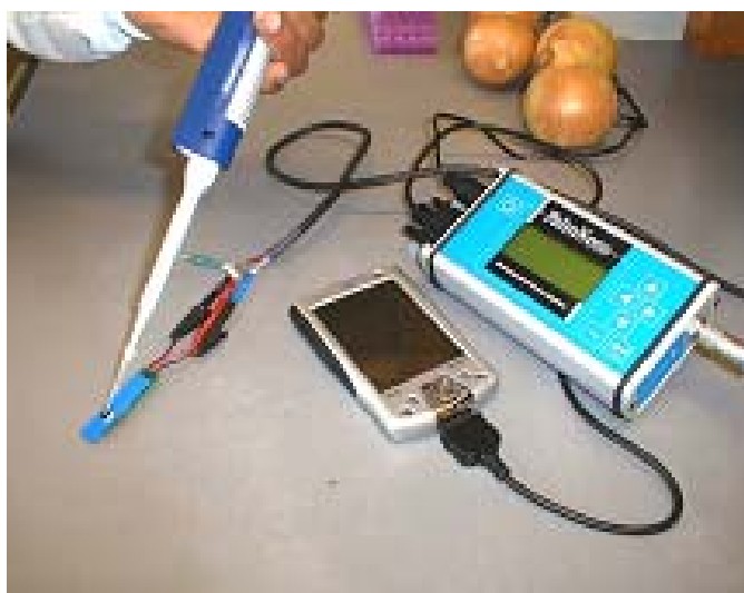
Plate 4.2. Experimental set-up: Portable potentiostat with three-electrode array
