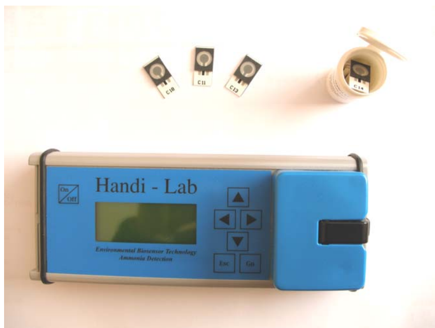
Plate 9.1. A Prototype transducer with disposable sensors. Reproduced with permission (Gwent Electronics Ltd, Pontypool, Wales, UK).
