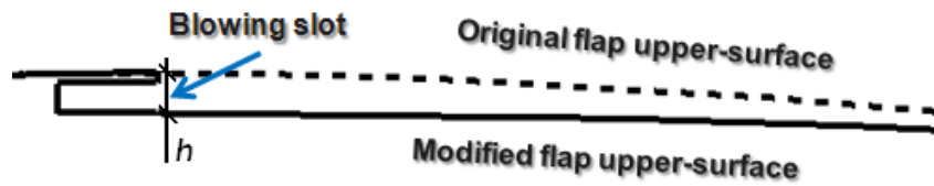
(b) Close up view of the blowing slot (Tangential blowing)
