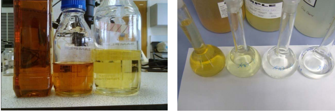
Figure 6-24: Left image; from left to right, Arpley treated landfill leachate, Arpley leachate following centrifugation, Arpley leachate following XAD-7 extraction. Right image; from left to right, MVP treated leachate, following centrifugation and XAD-7 extraction, following XAD-16 extraction, following XAD-4 extraction.
