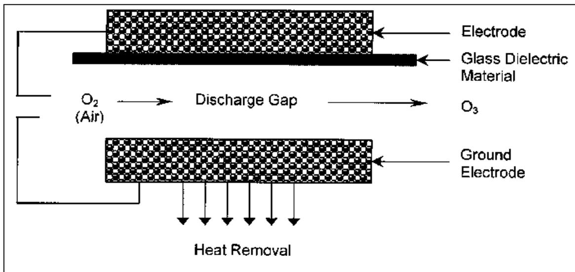
**Figure 1.5.** Schematic design of Corona Discharge (CD) ozone generation system (Muthukumarappan *et al.*, 2000).
