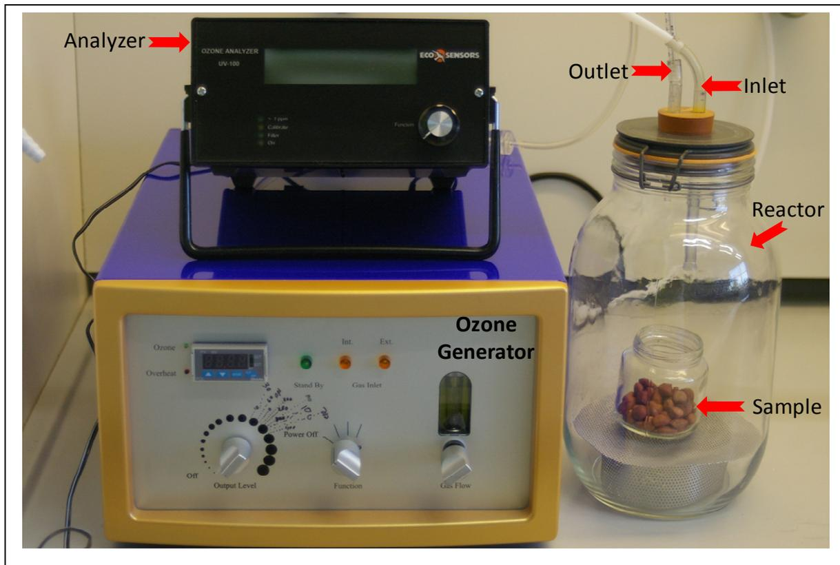
**Figure 4.1.** Set-up of the ozonation process including the O<sub>3</sub> generator, fumigation vessel and O<sub>3</sub> analyser.
