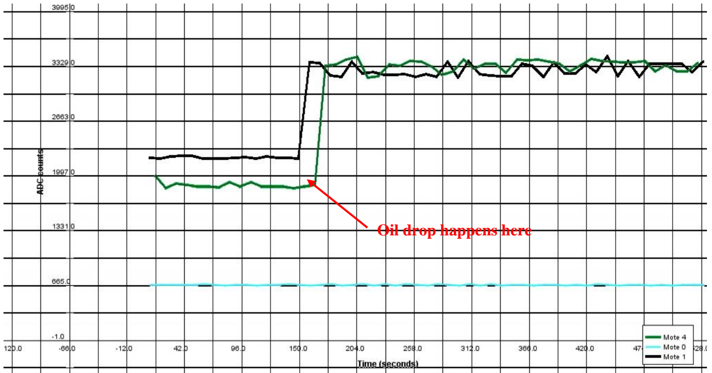
Figure 35. Oil detector sensor response when three motes are participating in the network.
