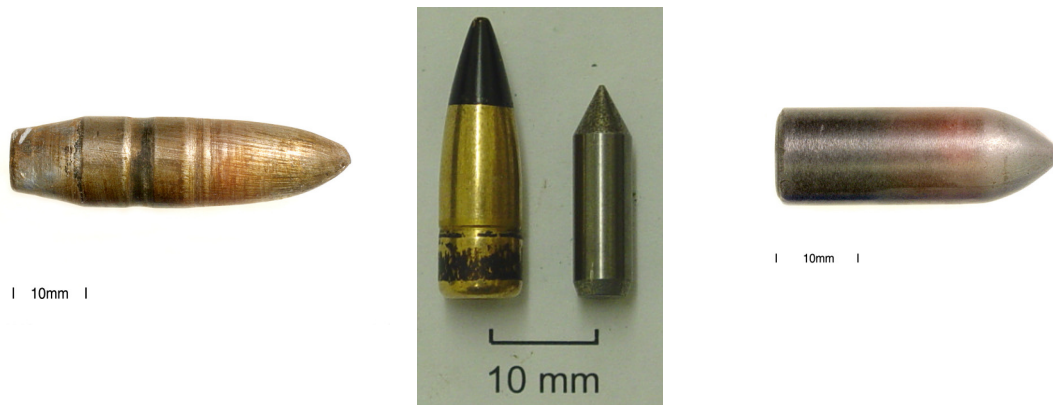
Figure A1.3: From left to Right: 14.5 mm B32 core, Bofors 7.62 x 51 mm FFV 1 , bullet and core, BS41 Core.
