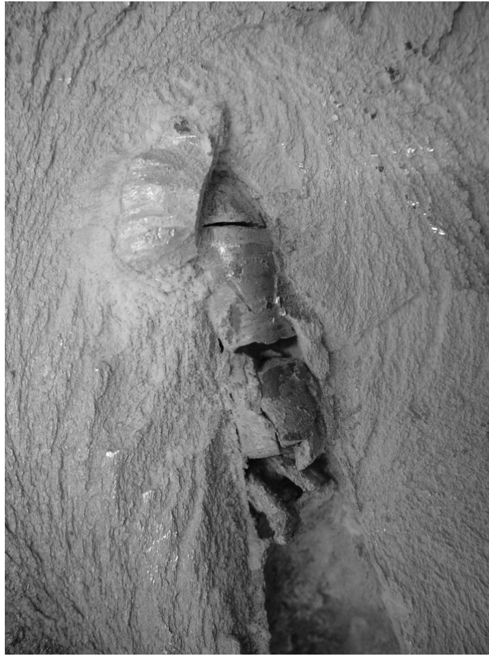
Figure 2.10: BS41 fractured WC-Co core. Captured by an 1318b aluminium alloy witness block after firing through a SiC B front face coupled to the 1318b aluminium alloy witness block.
