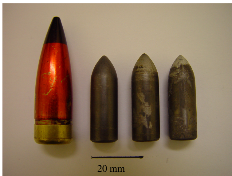
Figure 4.1: From left to right: BS41, BS41 unfired core, core retrieved after firing into mild steel and core retrieved after firing into 1318b witness block.
