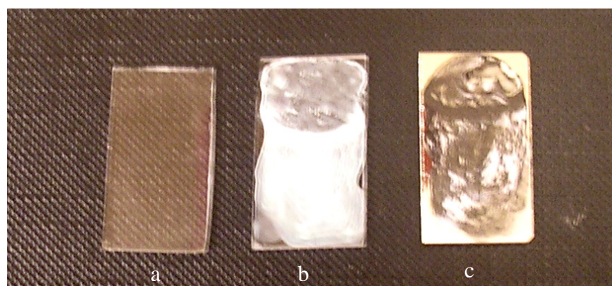
Figure 6.25 Surface fabrication process of a quartz-based surface with 60 nm silver layer coated at a 6^{\circ} slope. Quartz substrate (a) with a monolayer of the nanospheres (b) and after silver coating and the nanospheres removed (c).
