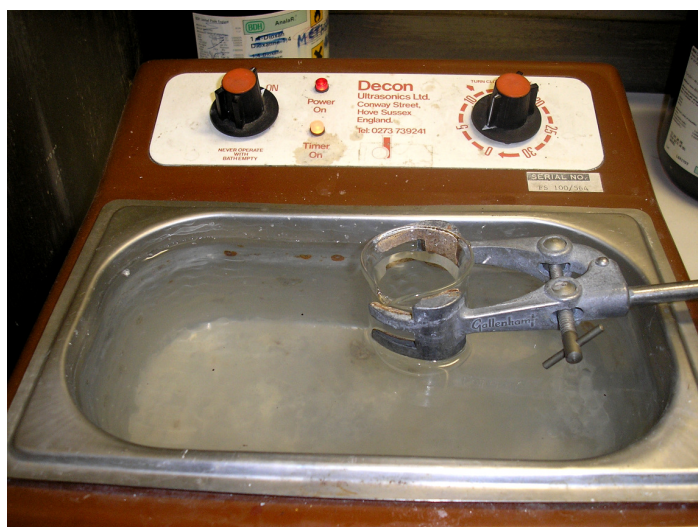
Figure 6.3 Removal of nanospheres by ultra-sonication in ethanol.
