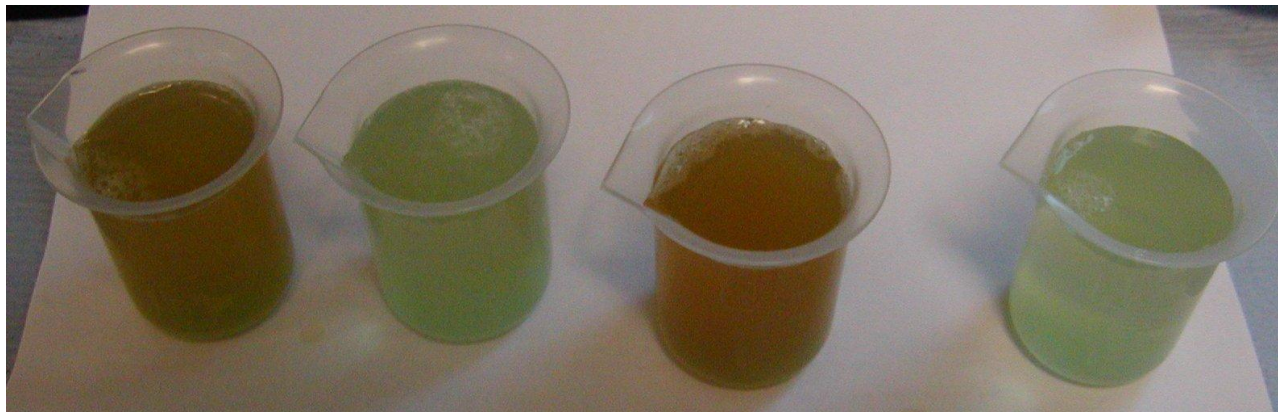
Figure 5.6: Photograph showing different buffers immediately after the addition of 26.6\text{mg}\cdot\text{ml}^{-1} iron (II) sulphate. From left to right the solutions are RO water, 10mM HEPES, 10mM TRIS, and 10mM MOPS all at pH 7.4.
