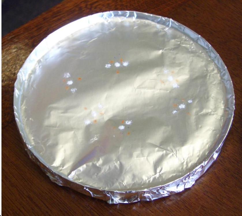
Figure 3.9: The foil coated lid of a petri-dish after a freeze-drying cycle, clearly showing material escaping the sample block wells and building up on the surface of the aluminium foil.
