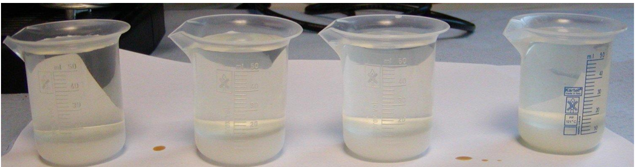
Figure 5.8: Buffer solutions after the addition of ascorbic acid at a concentration 20.6\text{mg}\cdot\text{ml}^{-1} . From left to right the buffers are: RO water, 10mM HEPES, 10mM MOPS, 10mM TRIS all pH 7.4.
