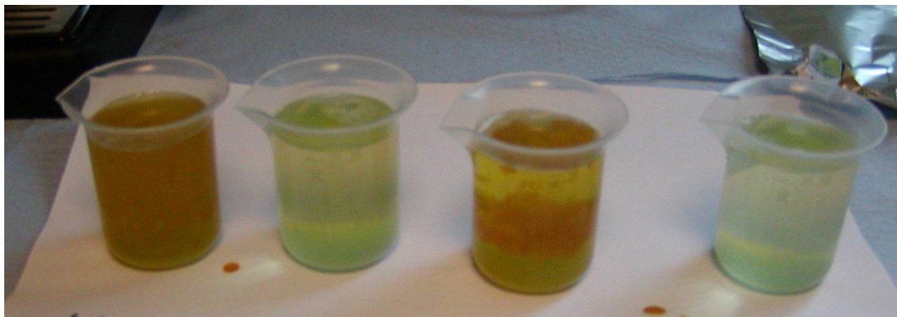
Figure 5.7: Photograph showing different buffers 1 hour after the addition of 26.6\text{mg}\cdot\text{ml}^{-1} iron (II) sulphate. From left to right the solutions are RO water, 10mM HEPES, 10mM TRIS, and 10mM MOPS all pH 7.4.
