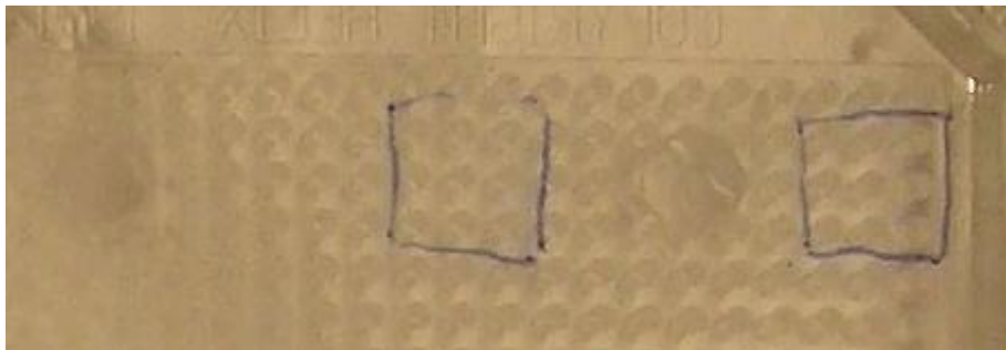
Figure 3.2: Customised 864 well microtitre plate with 9-well sample and control areas marked
