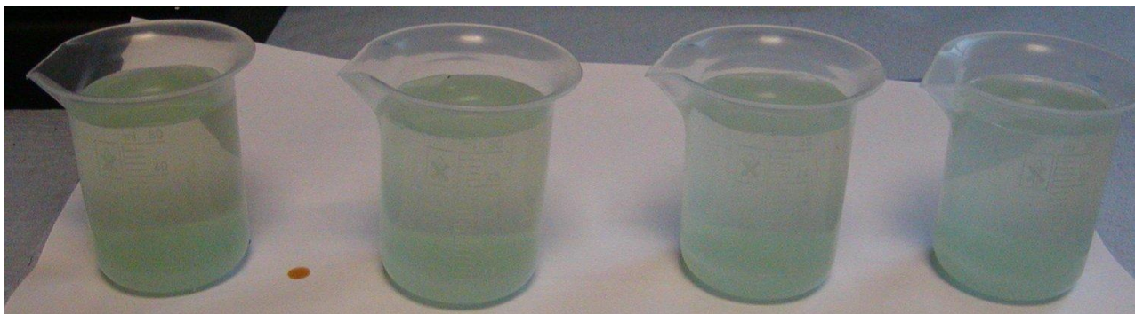
Figure 5.9: Buffer solutions containing ascorbic acid immediately after the addition of iron (II) sulphate at a concentration of 26.6mg.ml -1 . From left to right the buffers are: RO water, 10mM HEPES, 10mM MOPS, 10mM TRIS.
