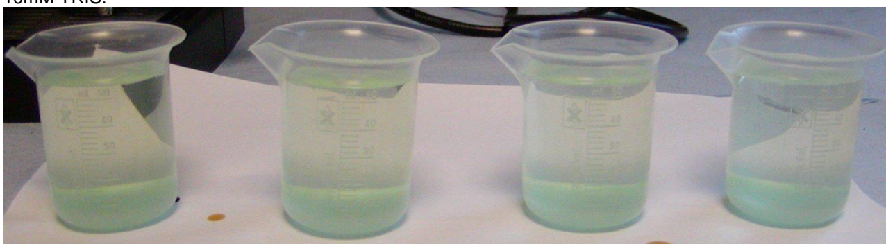
Figure 5.10: Buffer solutions containing ascorbic acid 1 hour after the addition of iron (II) sulphate at a concentration of 26.6mg.ml -1 . From left to right the buffers are: RO water, 10mM HEPES, 10mM MOPS, 10mM TRIS all pH 7.4.
