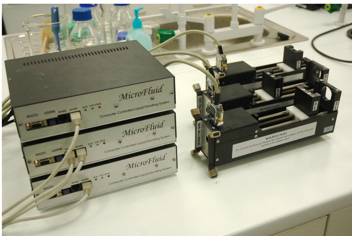
Figure 8.1 Custom-built precision syringe pusher: (left) controller; (right) syringe pusher.
