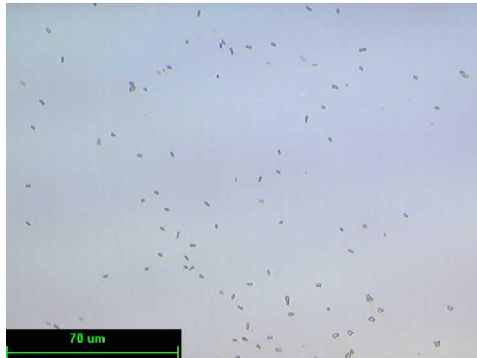
Figure 5.10 Optical micrograph of E. coli adsorbed on a \text{TiO}_2 waveguide.
