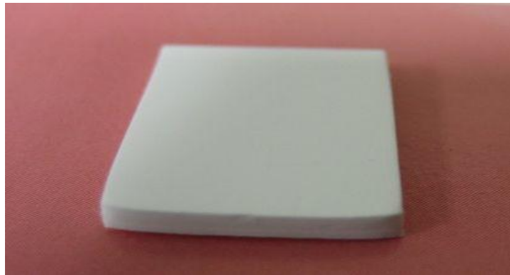
Figure 7.2 Teflon material ePTFE, 10 mm x 10 mm x 1mm.
