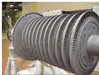
Fig. 4 Turbine rotor before it is placed inside the turbine housing.
