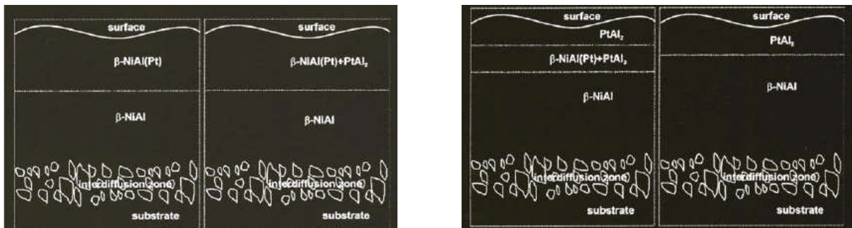
Fig. 20 a) Two profiles of a single-phase Pt-modified aluminide coating. b) Two profiles of a two-phases Pt-modified aluminide coating [30].
