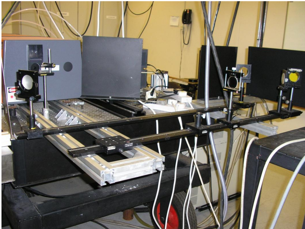
Figure 4.32: Optical arrangement for combined NO-PLIF and SPIV measurements
