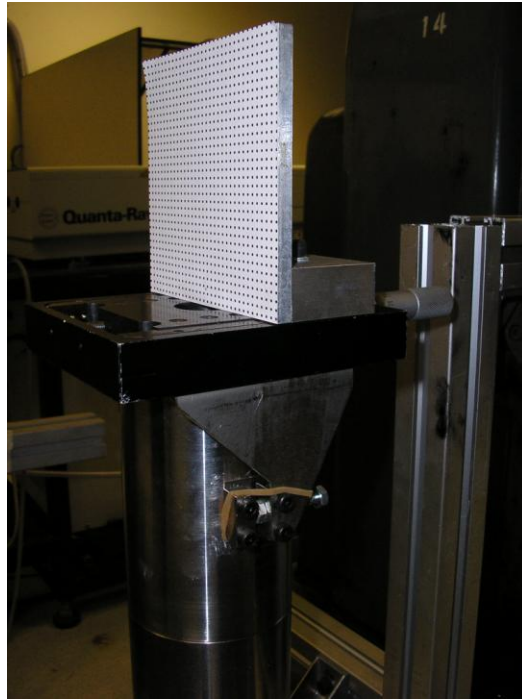
Figure 4.36: Calibration plate and its support used for the experiments
