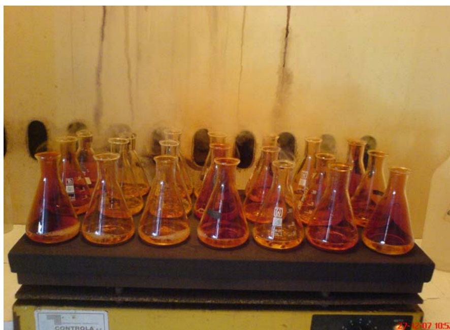
Plate A8. Digestion of samples on a hot plate inside the fume cabinet
