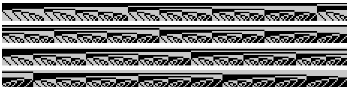
Figure D.2: Assigning data to test set or prediction set for cross-validation: Representation of 924 permutations for a selection of 6 out of 12, shown in four rows of 231 columns. Each column has 12 pixels (6 grey and 6 black). None of the 924 columns equal each other.
