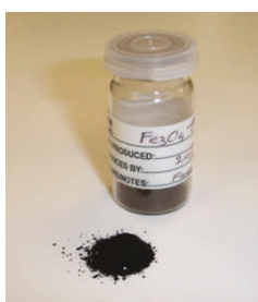
Figure 4.10: Black powder of synthesised \text{Fe}_3\text{O}_4 nanoparticles.
