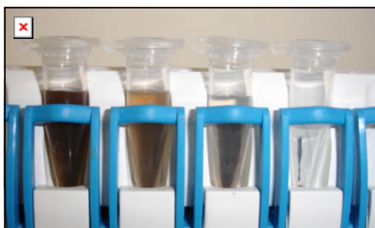
Figure 5.6: Photograph of nanoparticle-coated cells ( Rhodococcus erythropolis IGTS8) in Eppendorf tubes showing, successively: (A) dispersed cells coated with MNPs; (B and C) coated cells were gradually concentrated and collected towards the rear of the tube by an external permanent magnet (within the white housing behind the tubes); (D) liquid medium free of suspended NPs, which are visible as a thin dark stripe at the back of the tube.
