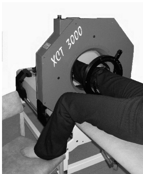
Figure 1: Set-up for lower limb bone scans using the pQCT scanner (XCT 3000, Stratec Medizintechnik, Germany).
