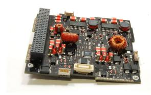
Figure 17 3U/2U CubeSat Power System.
