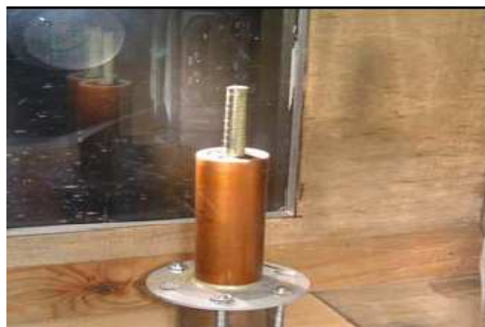
Figure 4-16: RAE/Plessey thermal probe
