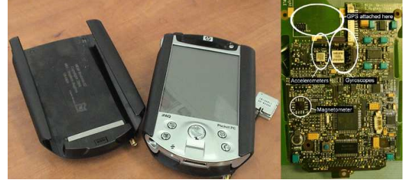
Figure 1: Left: Mesh device alone and attached to an HP5550 Pocket PC. Right: The MESH circuit board showing the main components related to the navigation task
