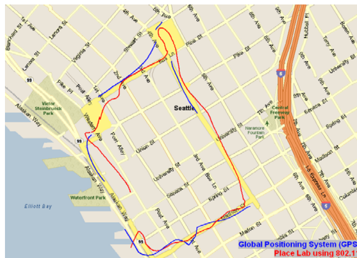
Figure 1. Place Lab and GPS are compared in this approximately 1km loop through downtown Seattle. The user started at the bottom and moved in a counter-clockwise direction around the loop. The red line is the series of location estimates based on wi-fi access points with Place Lab. The blue line is the series of location estimates from a GPS receiver – note the gaps in GPS coverage when the user rides a bus (on the left side of the loop) and enters a large shopping area (at the top).
