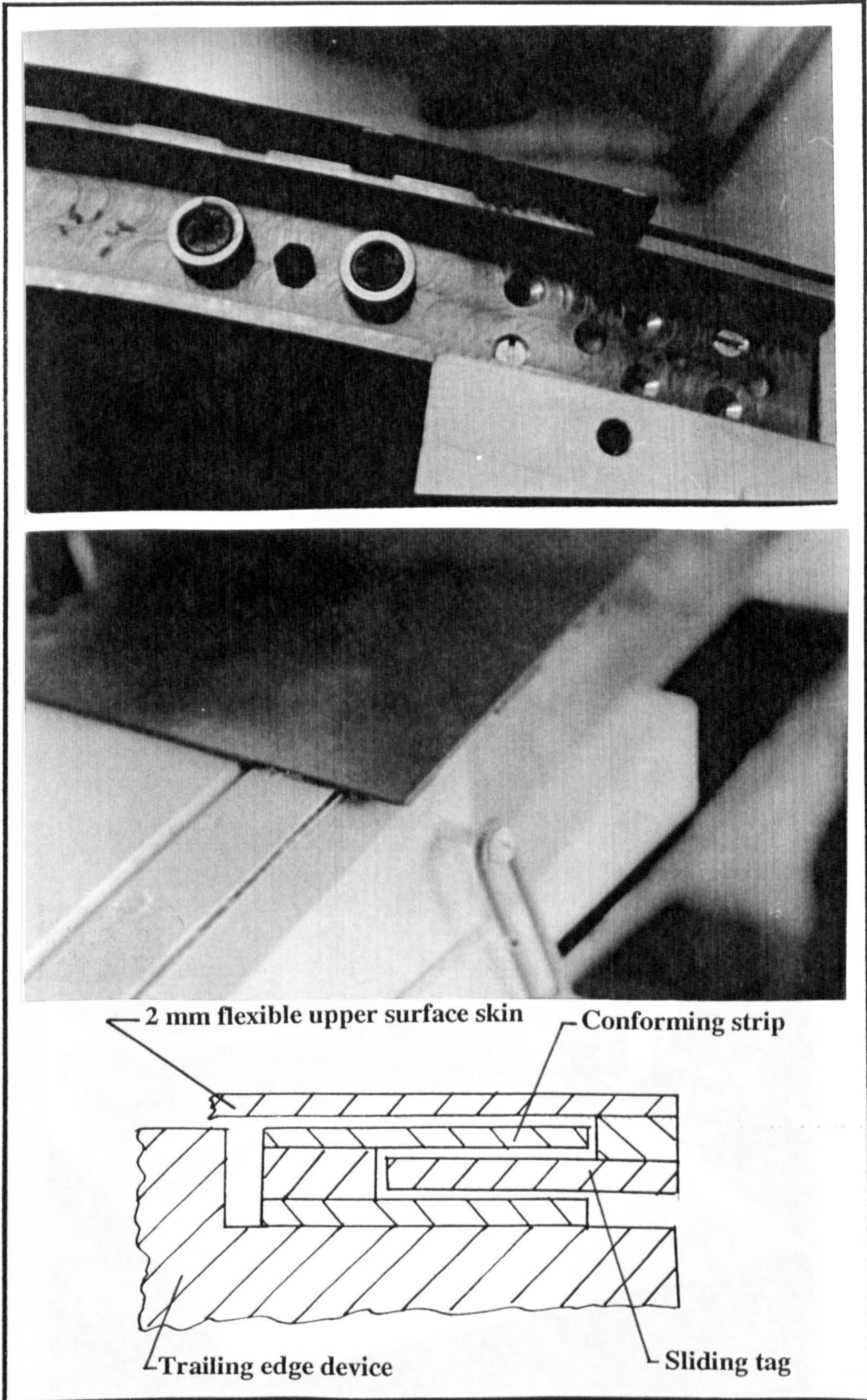
Figure 5.7: Solution for conforming the upper surface skin
