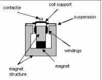
Figure 4: Typical construction of a voice-coil (shaker) transducer (adapted from [5]).
