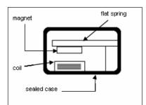
Figure 2: Construction of an inertial transducer similar to the TACTAID (adapted from [5]).
