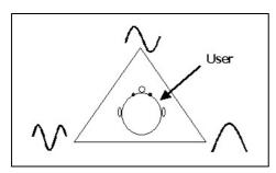
Figure 2: One series is positioned at each corner of an equilateral triangle, with the user in the centre
