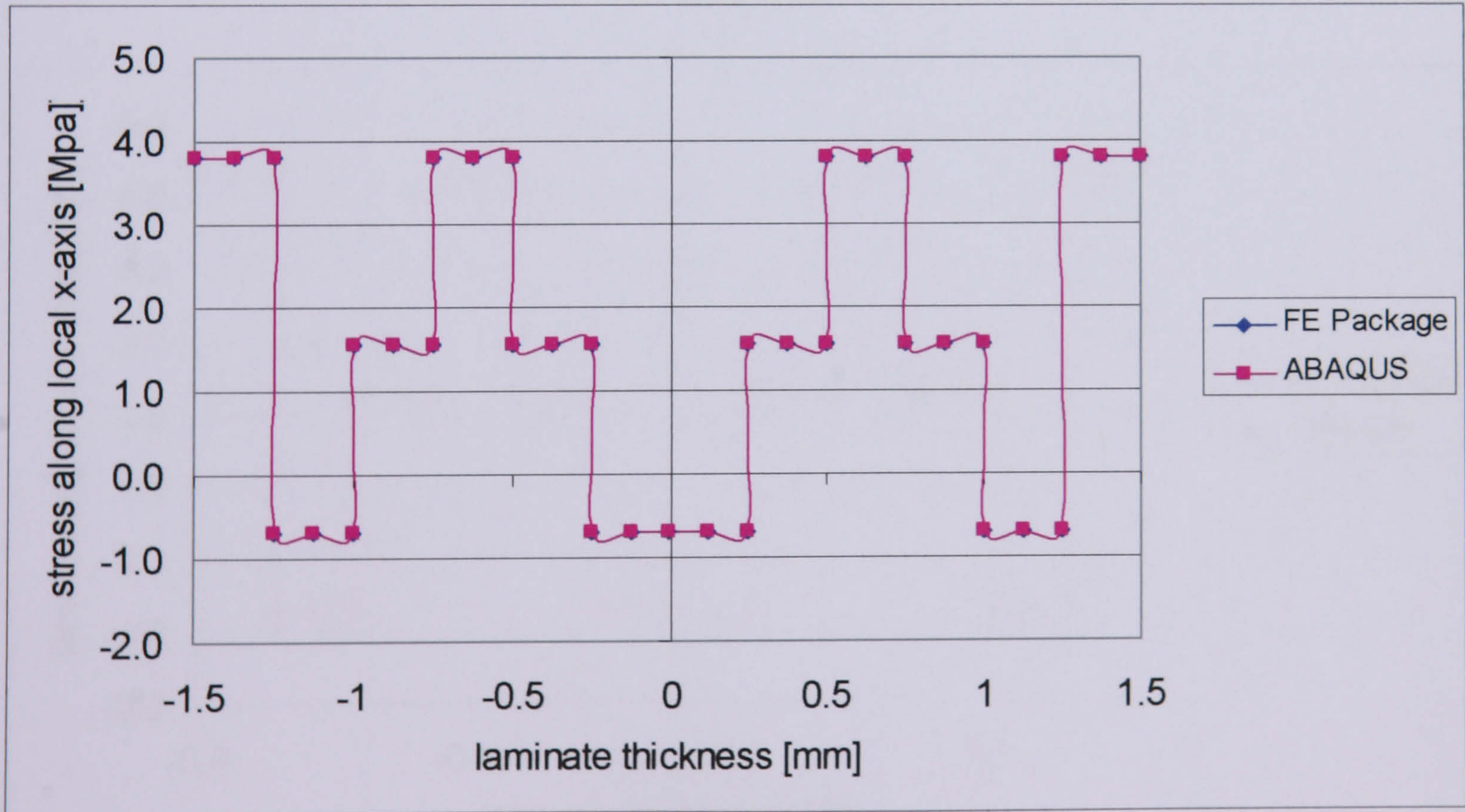
Figure (8.57) Axial stress ( \sigma_x ) distribution through the carbon/epoxy rectangular plate thickness at node 82.
