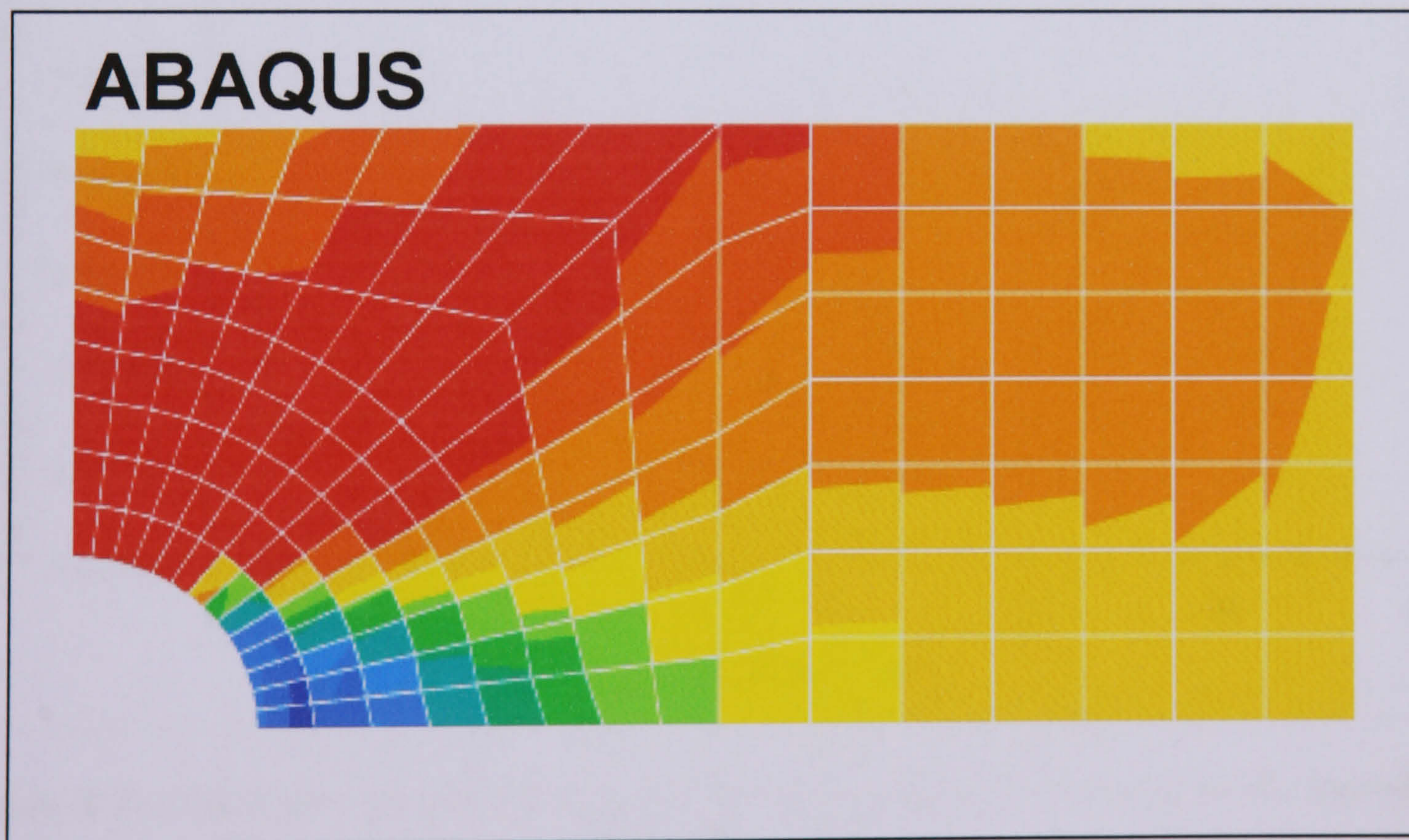
Figure (8.69) The damage zone of layer number two of the plate at the 23 rd iteration using the ABAQUS package.
