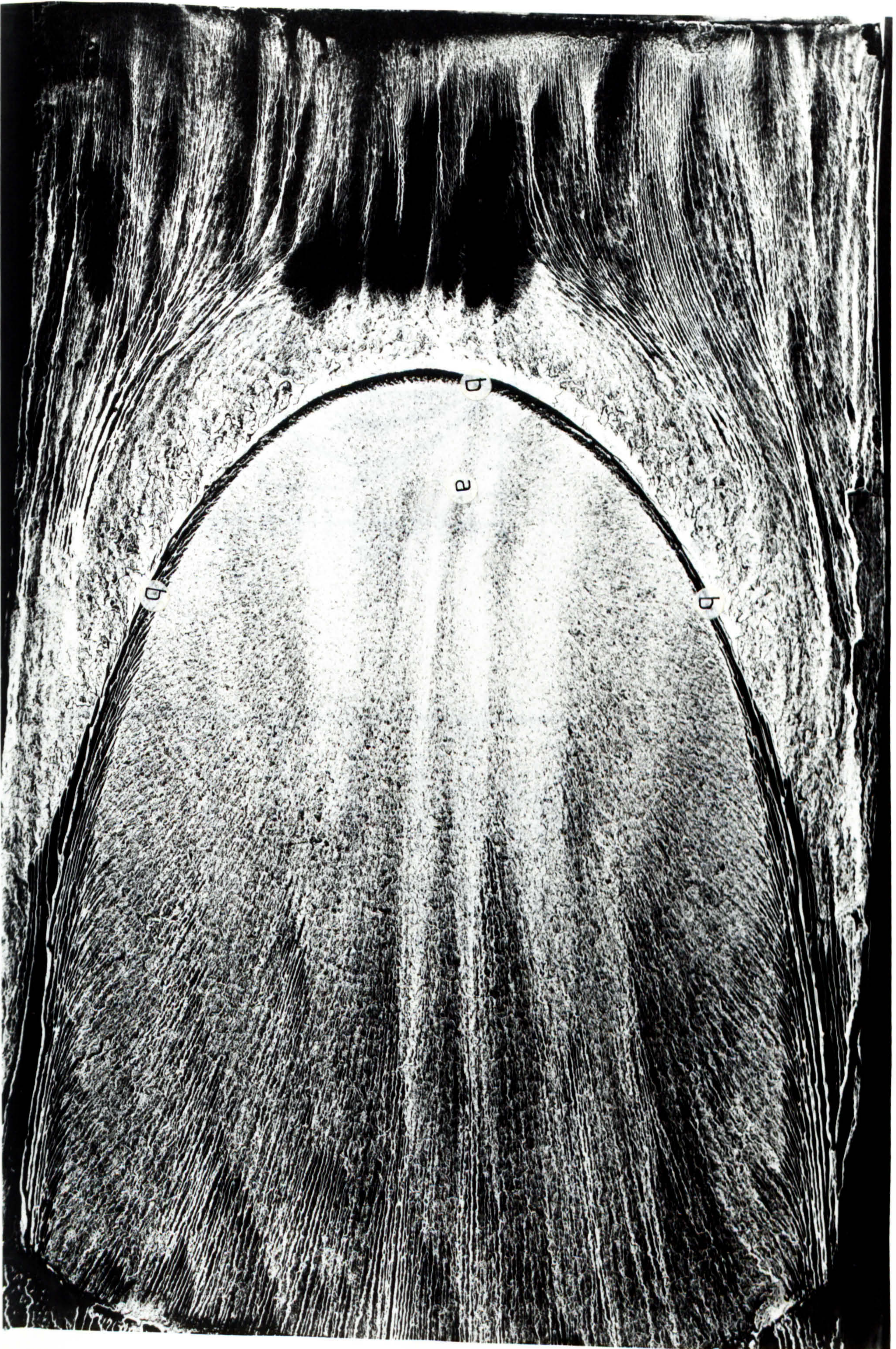
PLATE 8.2.1 SURFACE FLOW PATTERN ASSOCIATED WITH A CIRCULAR JET IN A CROSS FLOW (REF 36).
