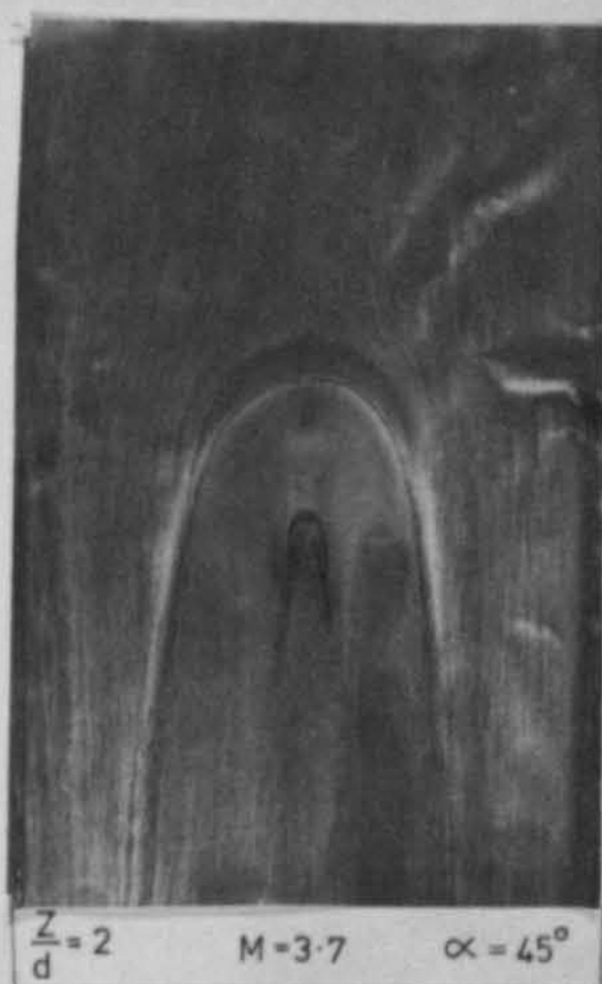
FIG. 7. 24. EFFECTS OF MASS VELOCITY RATIOS AND NOZZLE TO TARGET SPACING ON SURFACE FLOW PATTERNS ASSOCIATED WITH IMPINGING JETS IN CROSSFLOWS
