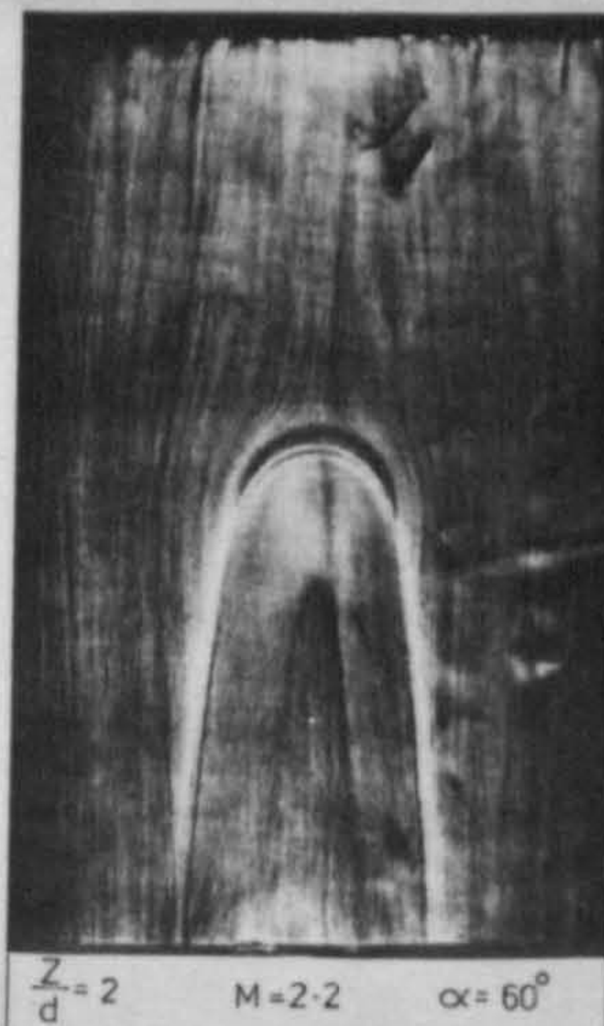
FIG. 7. 23. EFFECTS OF MASS VELOCITY RATIOS AND NOZZLE TO TARGET SPACING ON SURFACE FLOW PATTERNS ASSOCIATED WITH IMPINGING JETS IN CROSSFLOWS
