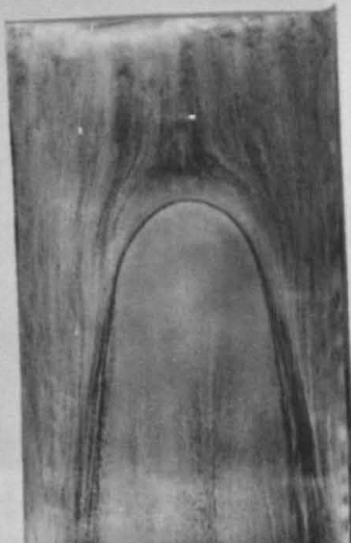
FIG.7.19. EFFECTS OF NOZZLE TO TARGET SPACING AND JET INCLINATION ON OIL FILM PATTERNS FOR IMPINGING JETS IN CROSSFLOWING AIR STREAMS
