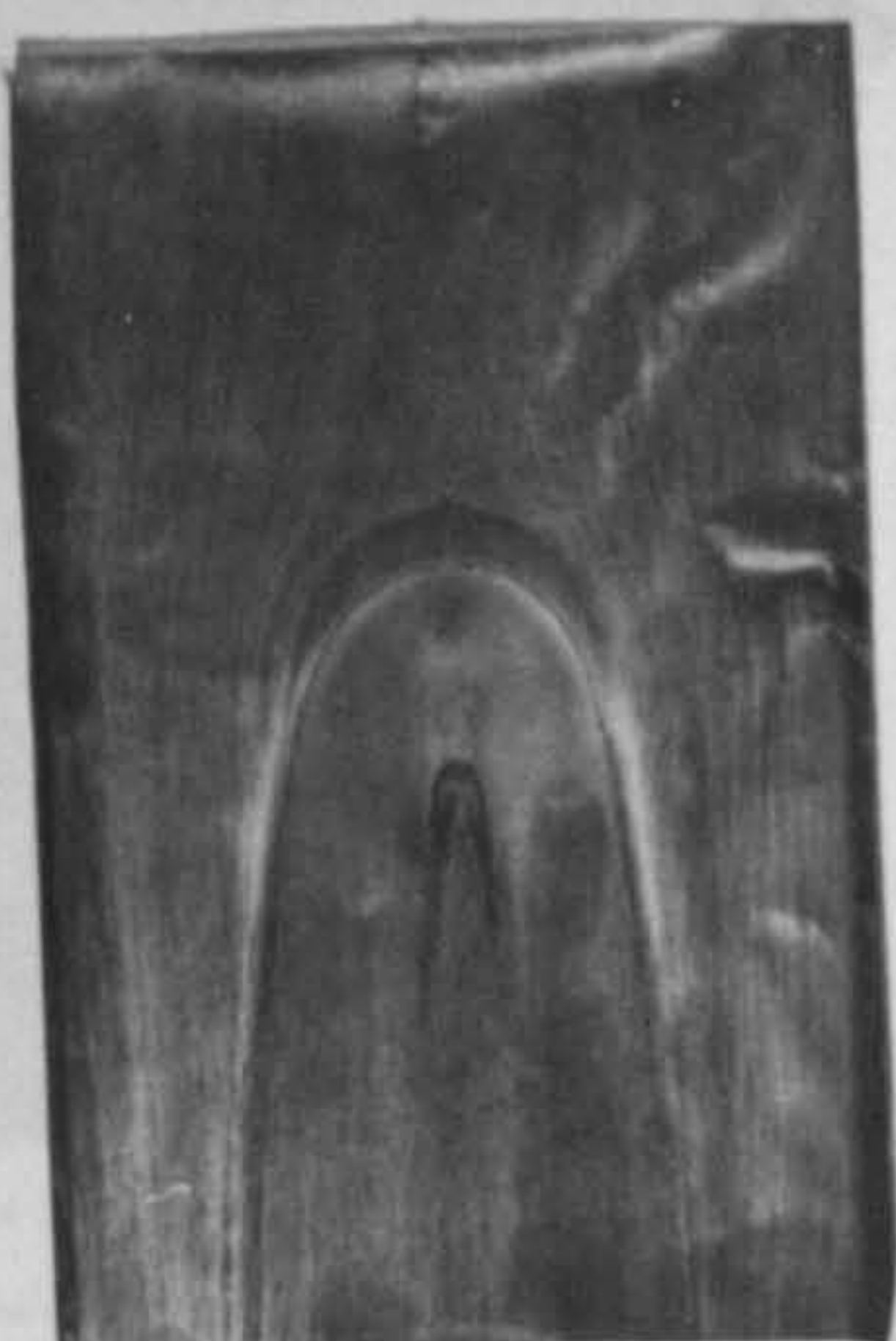
FIG.7.19. EFFECTS OF NOZZLE TO TARGET SPACING AND JET INCLINATION ON OIL FILM PATTERNS FOR IMPINGING JETS IN CROSSFLOWING AIR STREAMS
