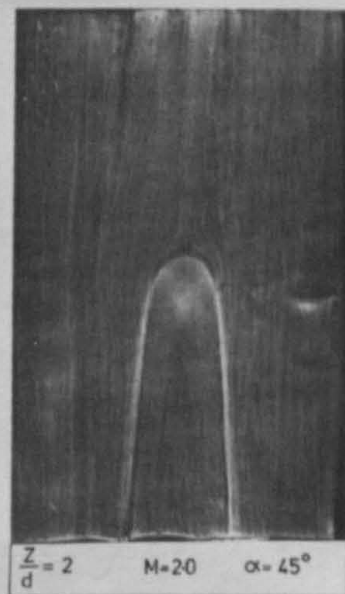
FIG. 7. 24. EFFECTS OF MASS VELOCITY RATIOS AND NOZZLE TO TARGET SPACING ON SURFACE FLOW PATTERNS ASSOCIATED WITH IMPINGING JETS IN CROSSFLOWS
