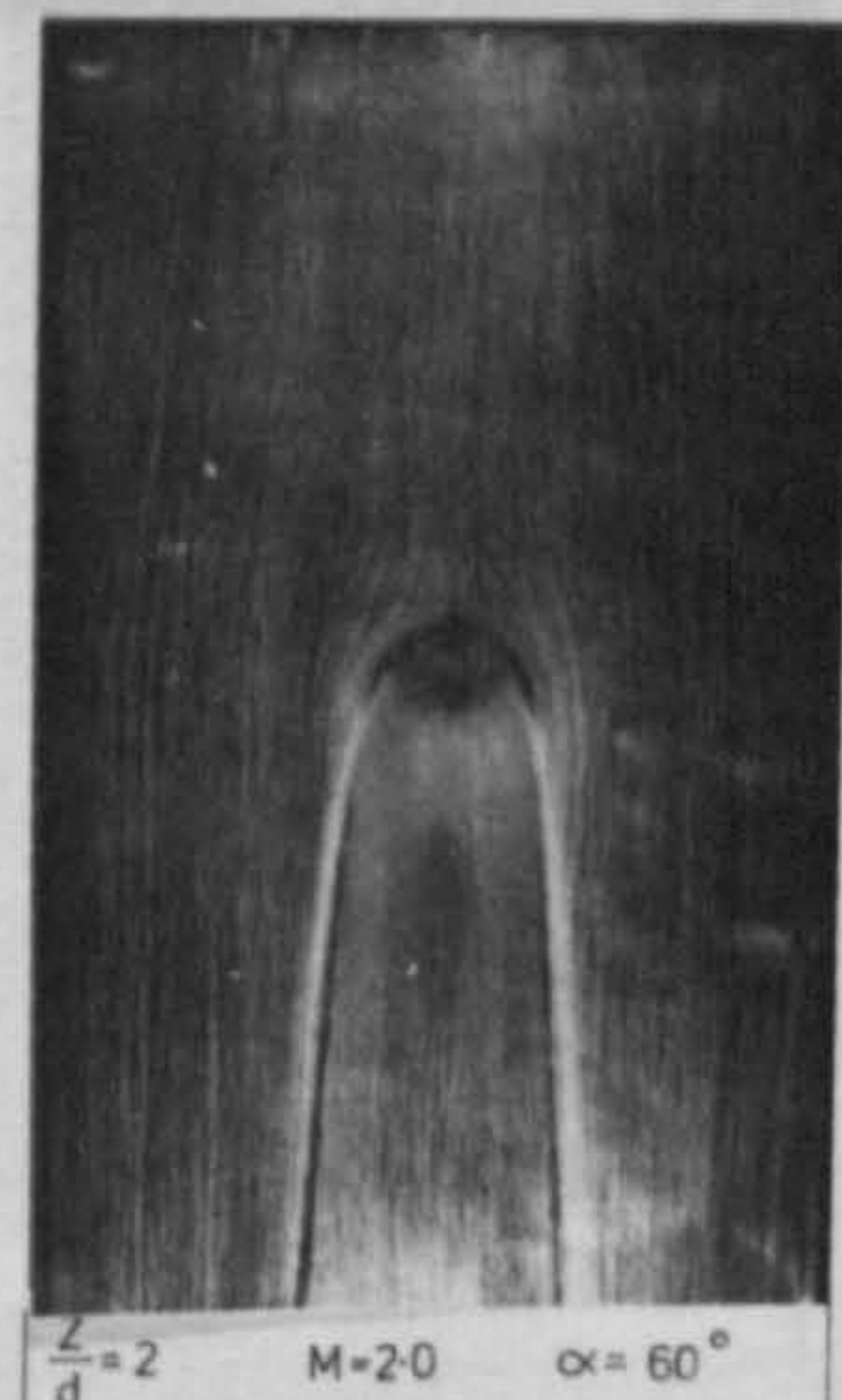
FIG. 7. 23. EFFECTS OF MASS VELOCITY RATIOS AND NOZZLE TO TARGET SPACING ON SURFACE FLOW PATTERNS ASSOCIATED WITH IMPINGING JETS IN CROSSFLOWS
