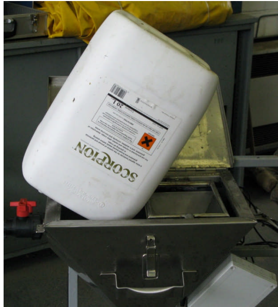
Figure 14: Modified induction hopper with a 20 litre container.
