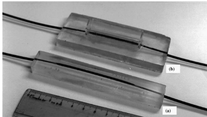
Figure 2.27 The POF sensor element manufactured by means of the side polishing technique on a resin block embedded fibre: (a) the sensor element; (b) the sensor element with a bonded cuvette around the exposed core. [62]
