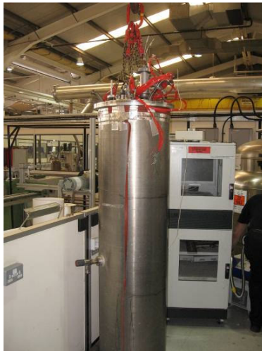
Figure 6.56 Cryostat containing prototype magnet.
