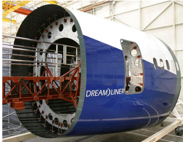
Figure 2.1. All composite fuselage section of Boeing Dreamliner [1].
