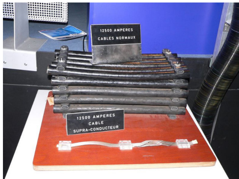
Figure 6.1 Superior current carrying capability of a superconducting cable when compared with conventional conductors.
