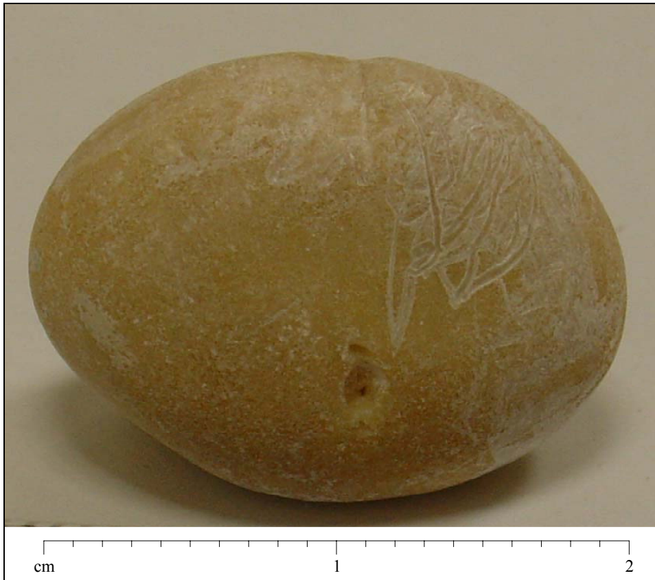
Figure 4.4: The photograph shows an intact specimen of a brushite calculus (calcium hydrate phosphate dihydrate). The crater seen at the front of the stone was caused by Nd:YAG laser irradiation during experiments described in a later section (see Appendix C for further details).
