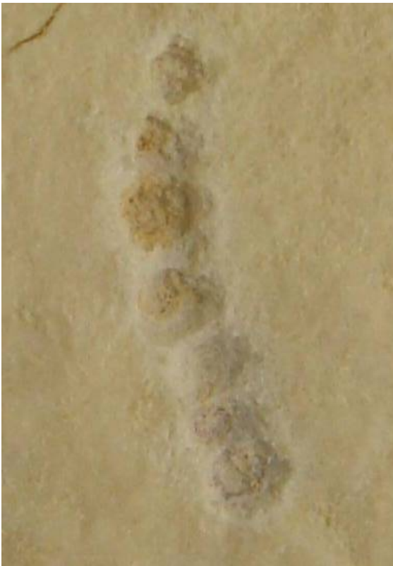
Figure C.4: Photograph showing a series of Ho:YAG laser-induced craters on a struvite calculus (Sample 3: magnesium ammonium phosphate hexahydrate) during irradiation in water. Each crater was formed by 10 laser pulses of \sim 1\text{J} per pulse. In this case, there is no apparent charring within the crater suggesting a dominant process of mechanical ablation i.e. possible shockwave action leading to stress fracture within the material. This is supported by the observation that crater size was estimated to be significantly larger than the fibre diameter; hence the action is not purely direct thermal ablation via a vaporised channel through water.
