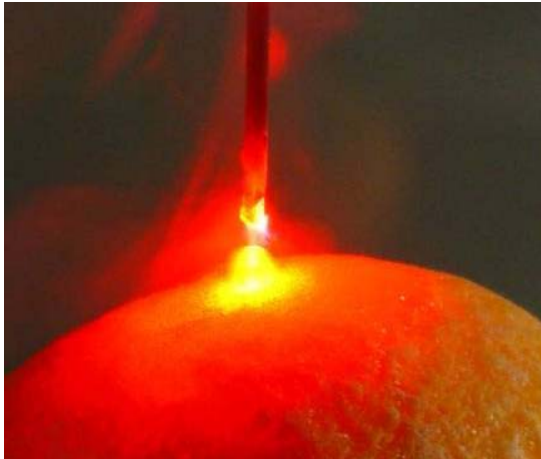
Figure 5.22: Photograph showing melting of cholesterol stone during holmium laser irradiation in air (Sample 13). Cholesterol has a melting point of \sim 150 °C.
