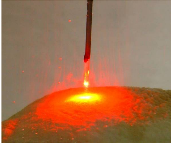
Figure 5.30: Photograph of Ho:YAG laser action on a urinary calculus in water. The calculus shown is mainly composed of struvite (Sample 3).
