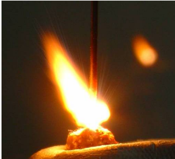
Figure 5.20: Photograph capturing the thermal interaction of pulsed holmium laser on a uric acid calculus in air (Sample 3).
