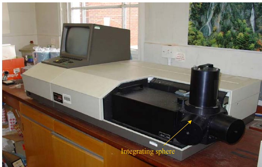
Figure 4.32: The Lambda 9 system used for diffuse reflectance measurements
