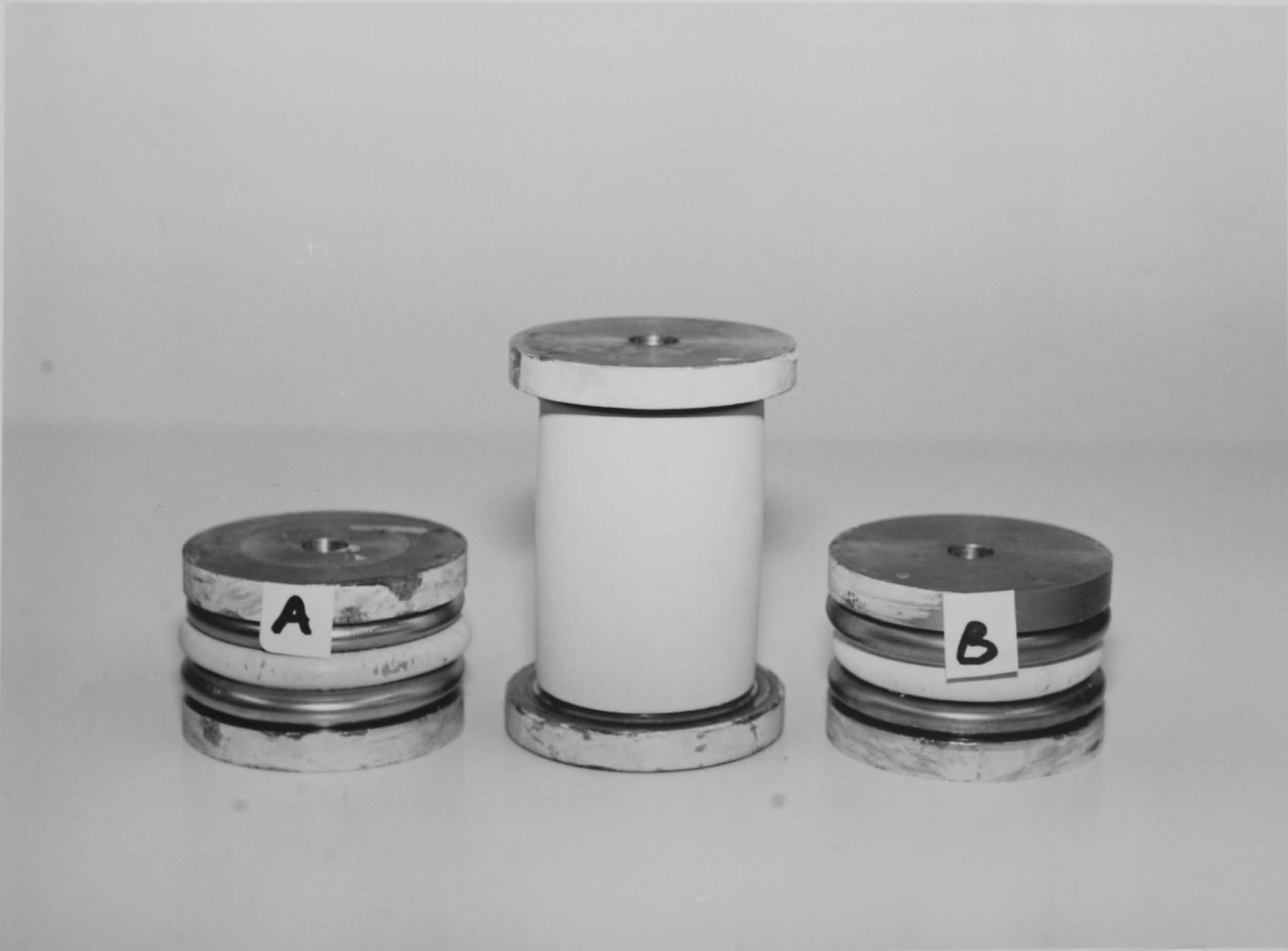
Fig.2.11 Inverbucktubes before and after collapse
