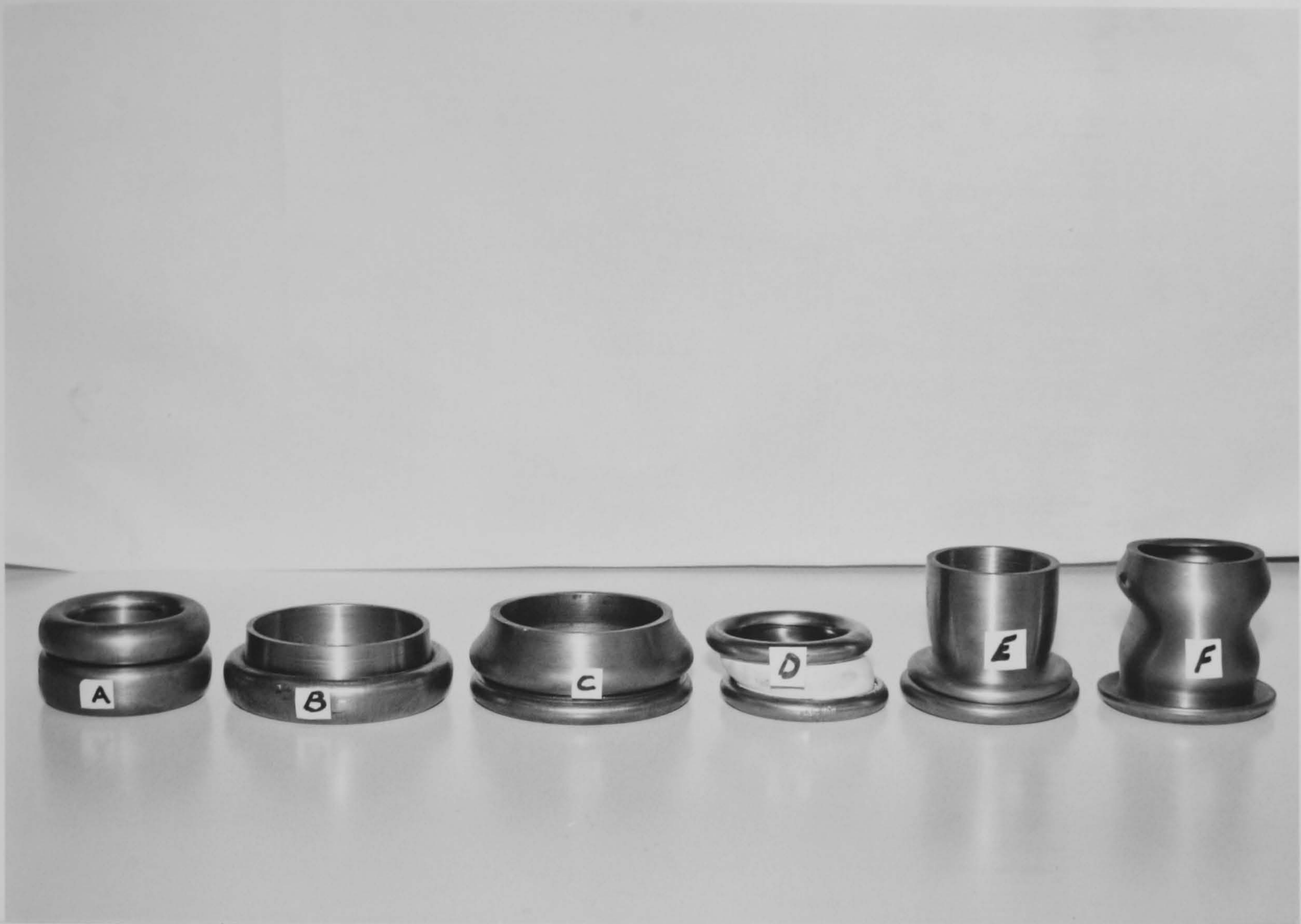
Fig.2.10 Possible modes of deformation depending on \bar{D}/2t_A
