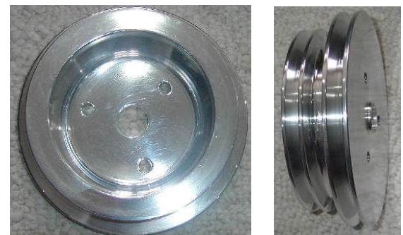
Figure 8: New pulley to drive the water pump and power steering pump – CAD model and machined part.
