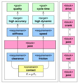
Figure 7: Simplified example of the hierarchical view on requirements of components (left) and component structure in a kinematic chain (right).
