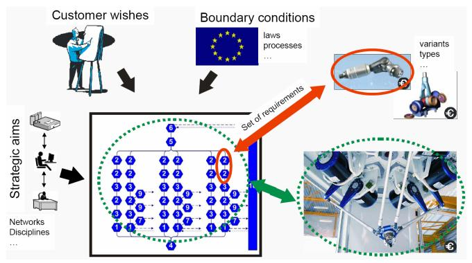
Figure 3: Requirements and constraints for the parallel robot HEXA (schematic overview).
