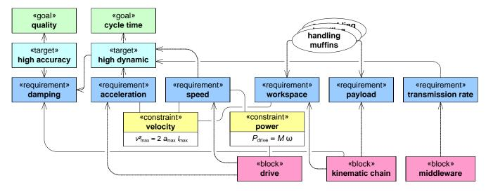
Figure 6: Goal oriented view on the product, excerpt of an extended requirements diagram based on SysML.
