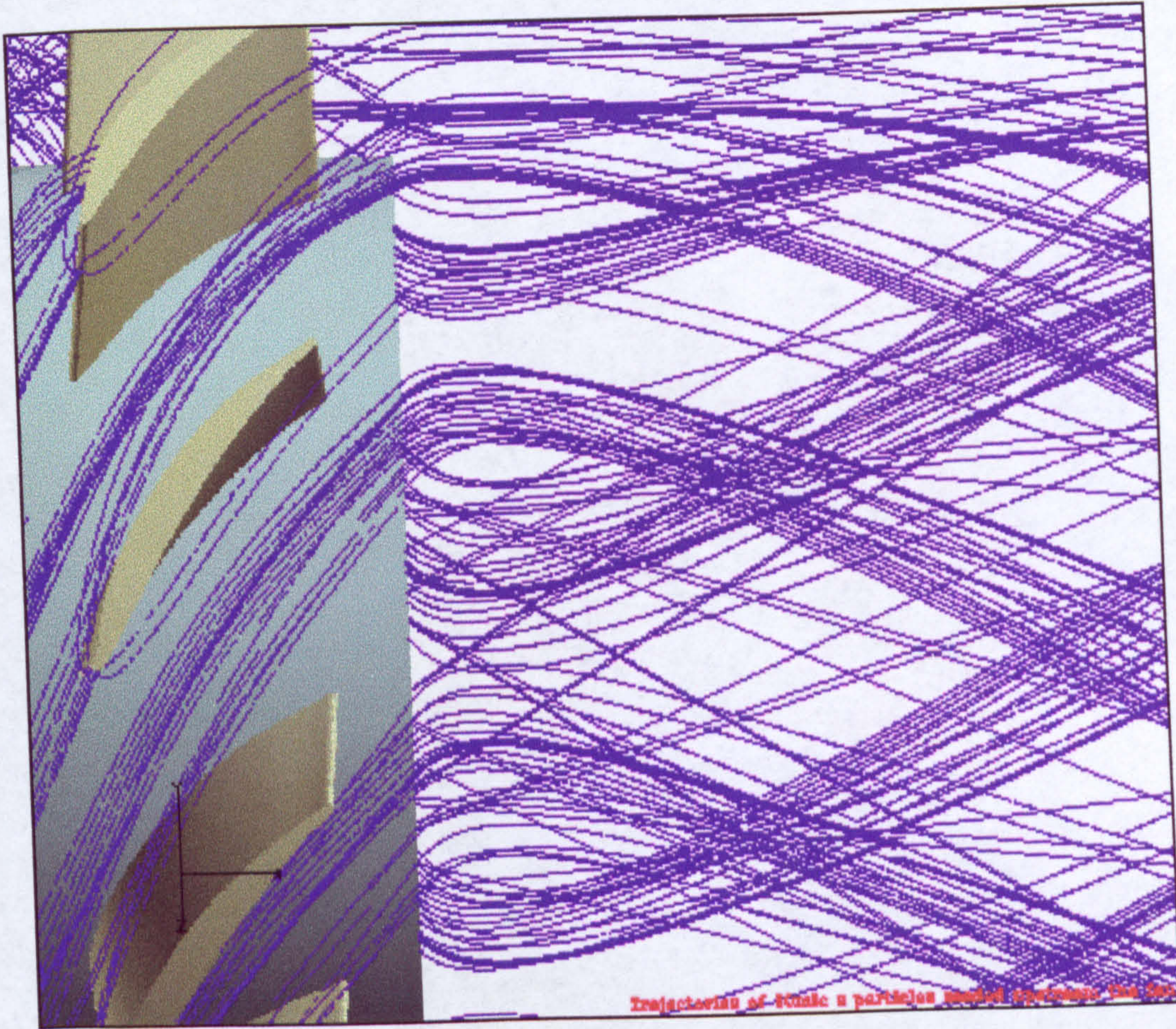
Figure 3-31 Trajectories of fine particles between rotor blades
