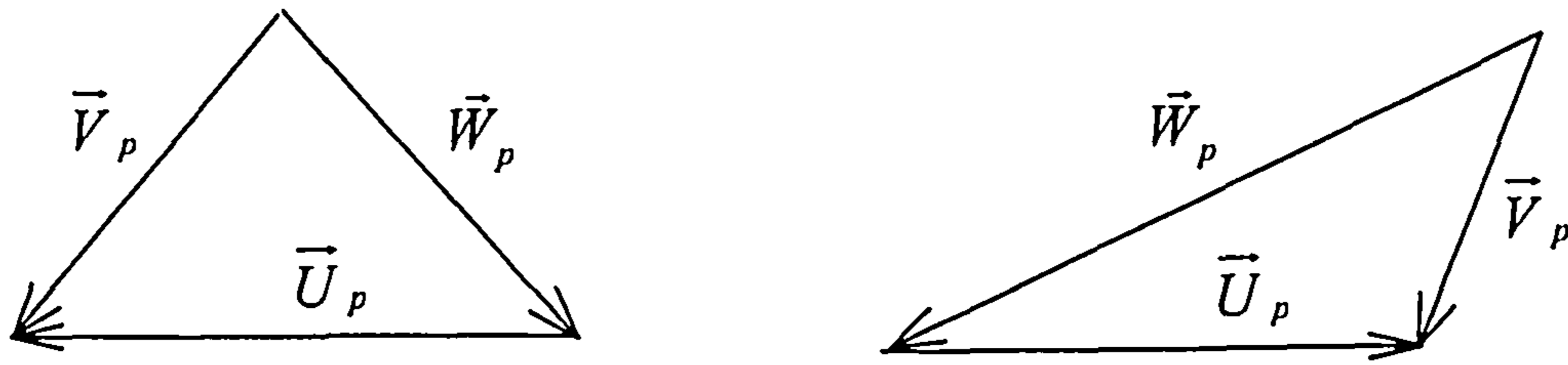
Figure 3-2 Velocity triangle across an interface plane
