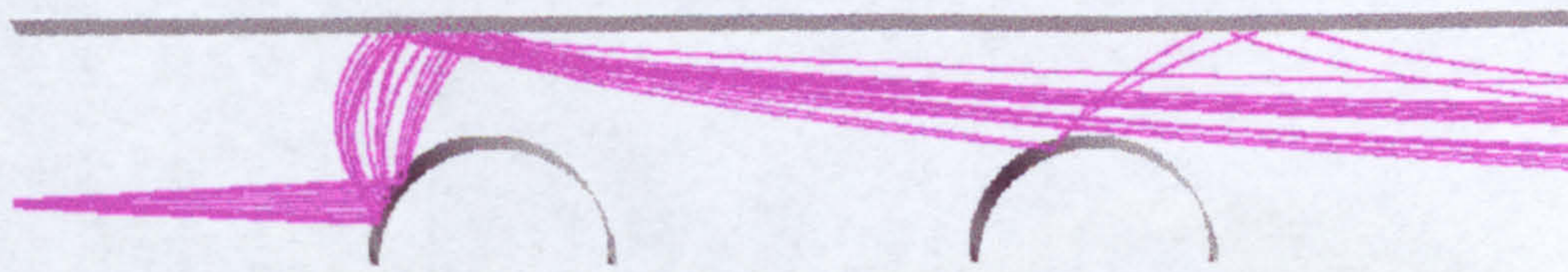
Figure 3-17 Trajectories of sand particles (150-300 micron) seeded upstream locally
