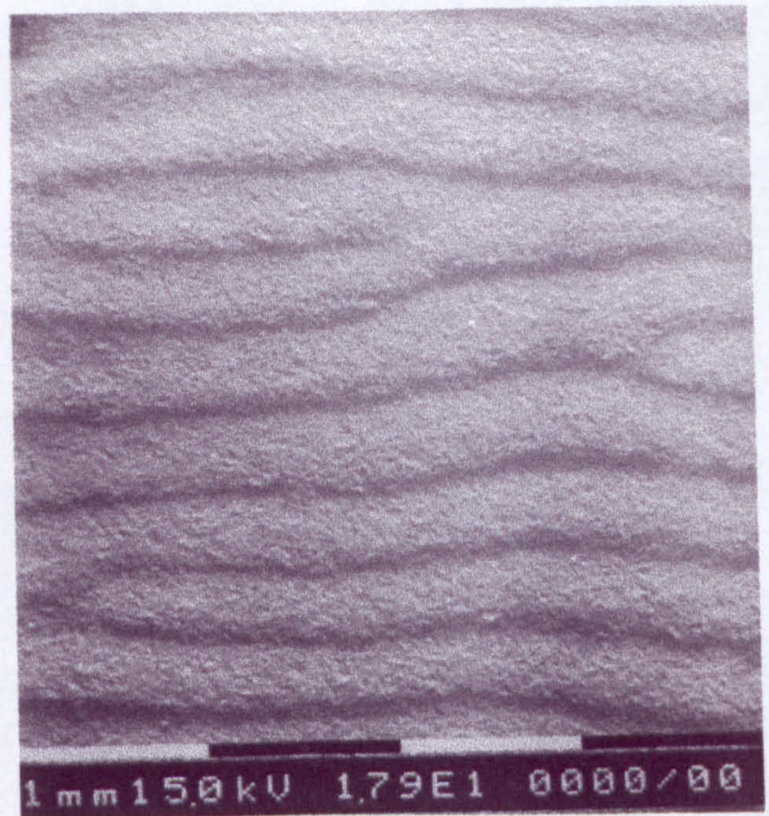
Figure 4-8b Scanning electron micrographs of eroded cast aluminum at angle 40 degree
