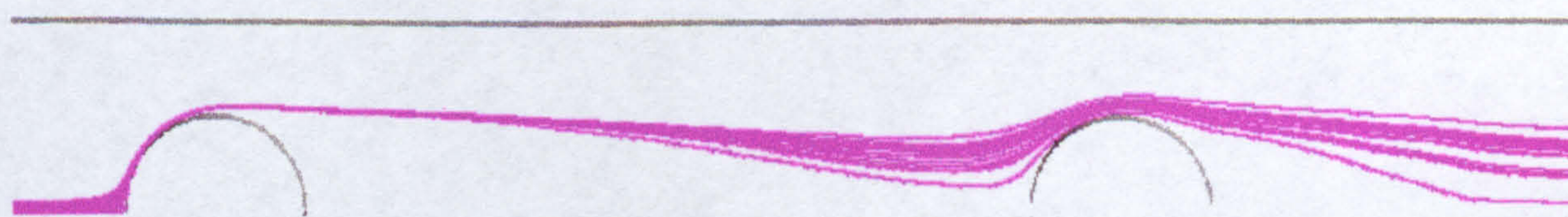
Figure 3-20b Trajectories of 10 micron around half tandem cylinders considering turbulence
