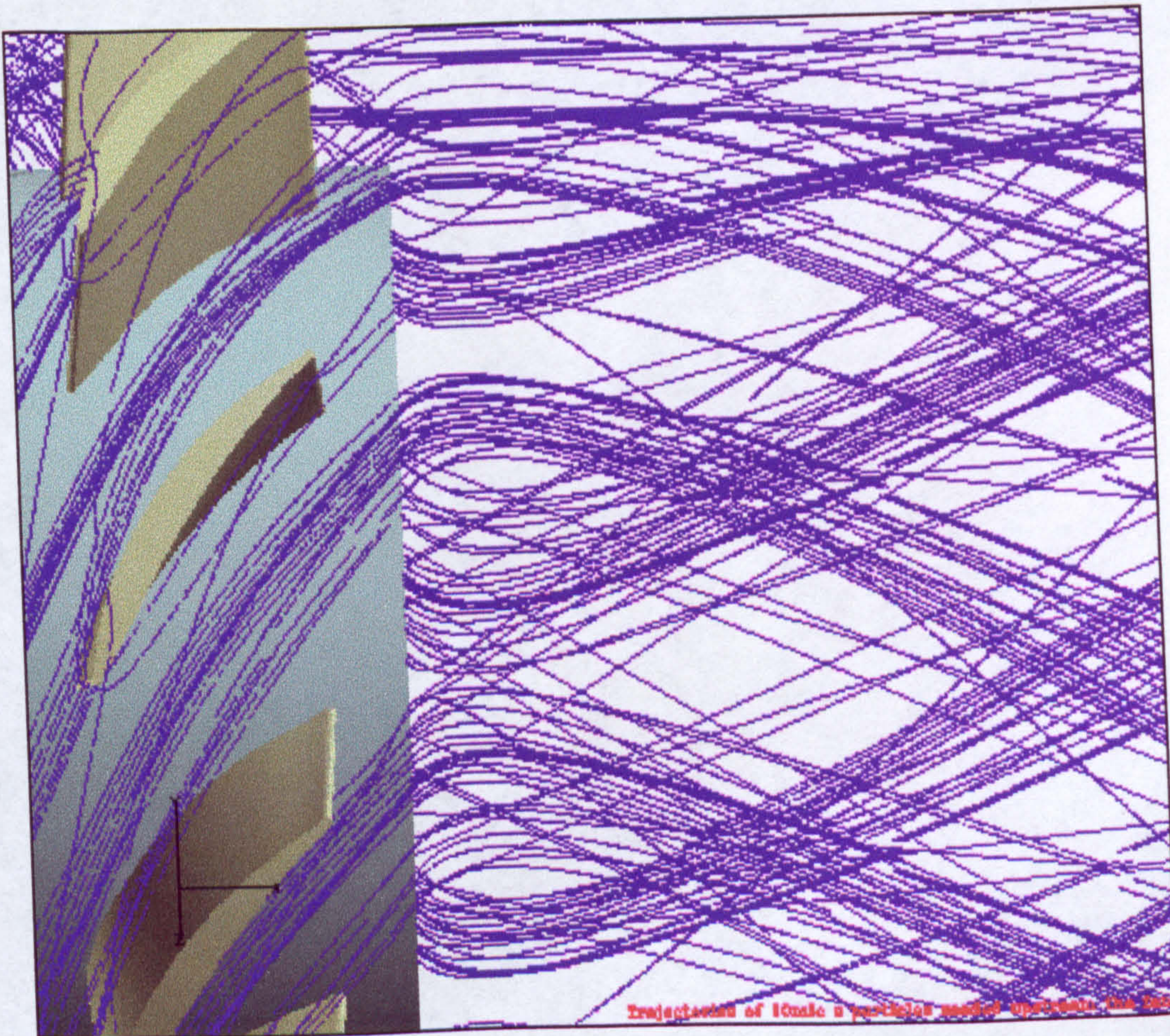
Figure 3-32 Trajectories of fine particles between rotor blades considering turbulence
