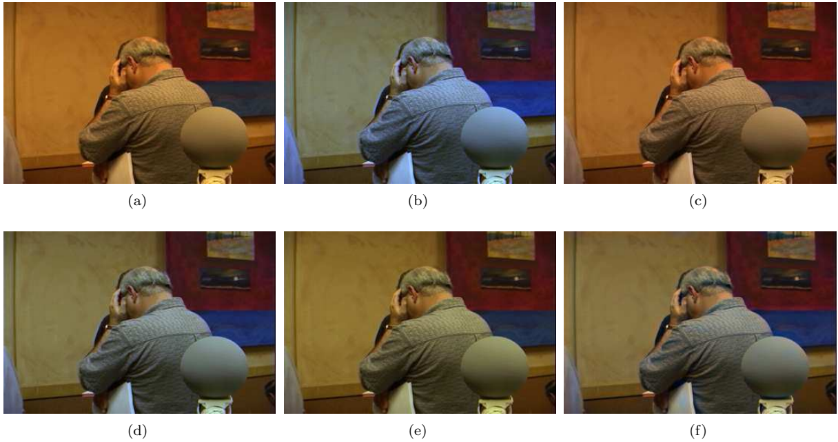
Figure 7: Colour constancy results and the corresponding angular errors between estimated and ground-truth illuminant colours using different algorithms on an input image from the Grey Ball dataset [20]. (a) Input image. Illuminant-colour corrected images obtained using: (b) Grey-World ( \Delta\theta = 7.6^\circ ); (c) Max-RGB ( \Delta\theta = 14.7^\circ ); (d) Shades of Grey ( \Delta\theta = 3.0^\circ ); (e) Grey-Edge ( \Delta\theta = 8.1^\circ ); and (f) proposed algorithm ( \Delta\theta = 1.6^\circ ).
