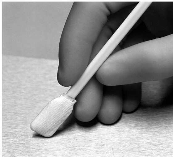
Figure 2.3. Showing the removal of samples from surfaces with a swab for subsequent analysis. Source: Miscoscio, 1997.
