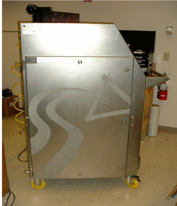
Figure 2.7. The ePAT 731 analyser manufactured by Expo technologies.
