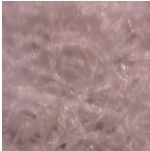
Figure 3.5. Showing fibres from a Technicloth™ swab (x 20).
