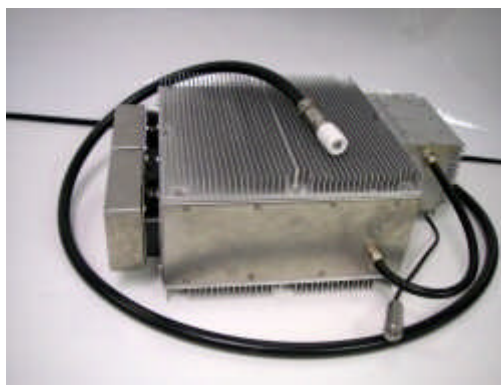
Figure 2.6. The ePAT 631 analyser manufactured by Expo technologies.
