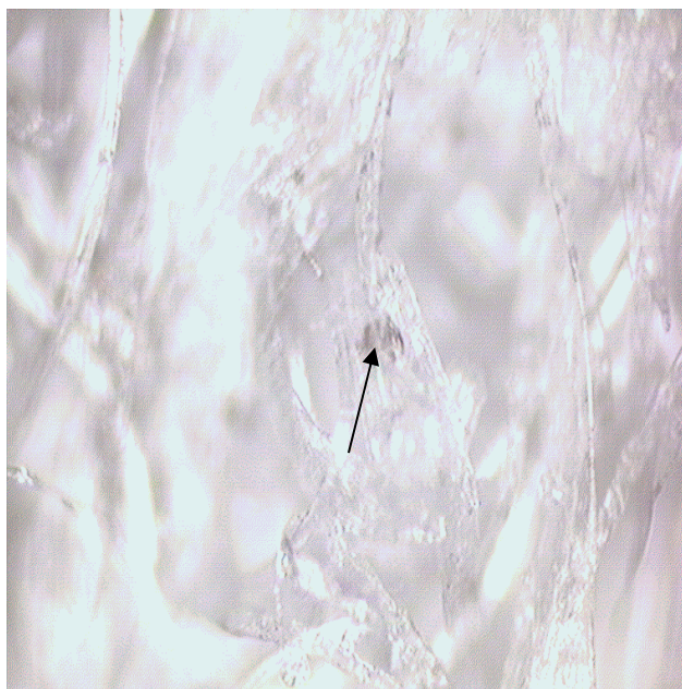
Figure 4.38. An image taken of a gold colloid impregnated Texwipe™ swab (x10). The area indicated by the arrow in the centre of the image is an aggregation of gold particles. There are other smaller clusters of gold aggregate in the image. SERS spectra are obtained from these swabs by focusing the laser on areas containing aggregated gold particles.
