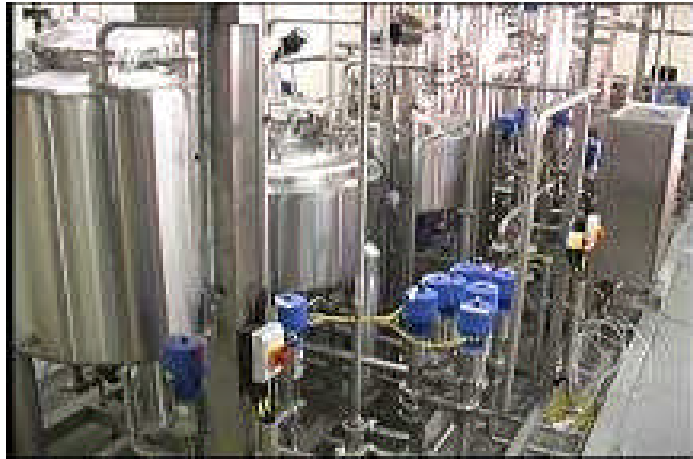
Figure 1.1. Photographic example of a pharmaceutical pilot plant. The presence of large surface area, plus pipes, valves etc means that cleaning is an arduous process and it must be done rigorously to ensure that residues are eliminated.
