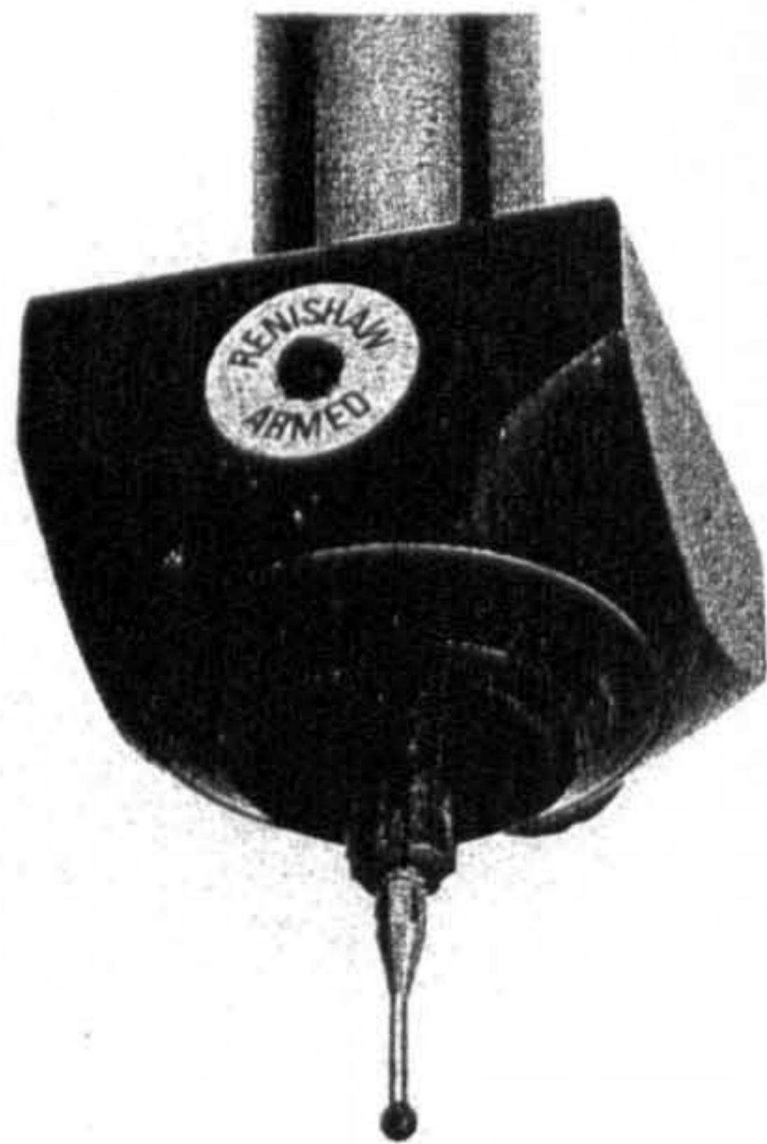
Early touch-trigger probe
