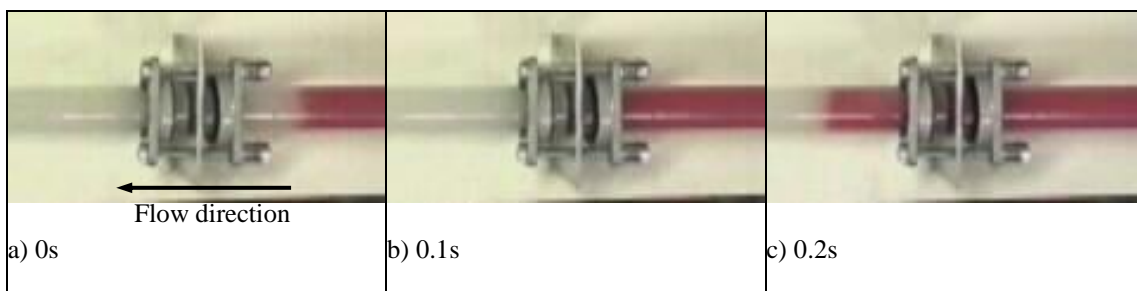
Fig. 5. Passage of 60 % ice slurry through an orifice at a flow velocity of 0.4 m/s.
