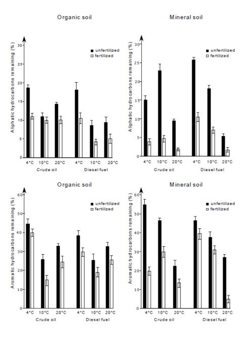
**Table 1:** Changes in oil hydrocarbon fractions concentration (as % degradation of initial value) over 180 days. Each percentage represents the mean of hydrocarbons fractions from duplicate samples
