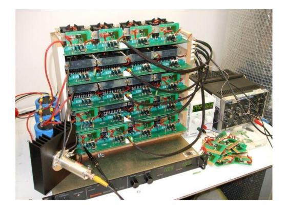
Fig. 2(a). The custom-built repetitive avalanche test equipment capable of testing 16 MOSFETs simultaneously.
