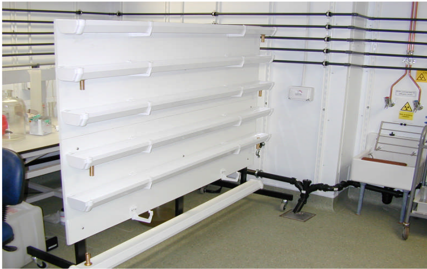
Plate 4. Artificial river model system, consisting of five channels.
