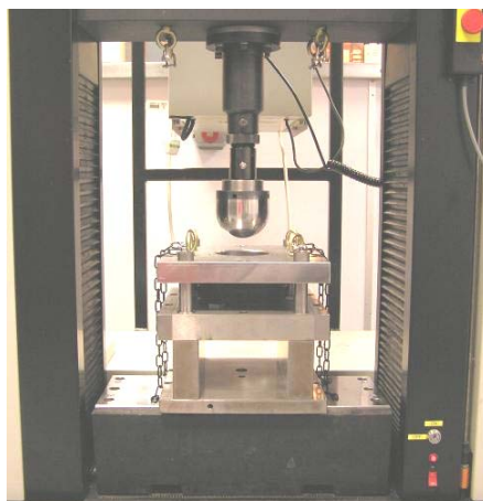
Fig.3 Experimental setup showing LDH tooling installed on an Instron
