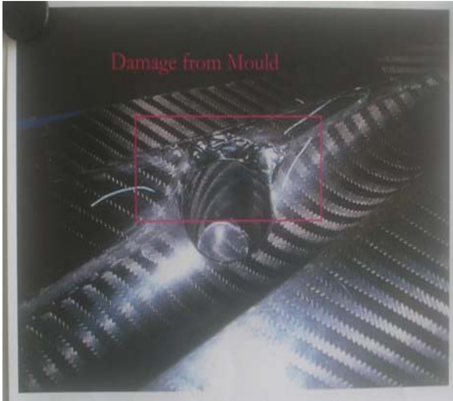
Figure 11: Damage from Mould
